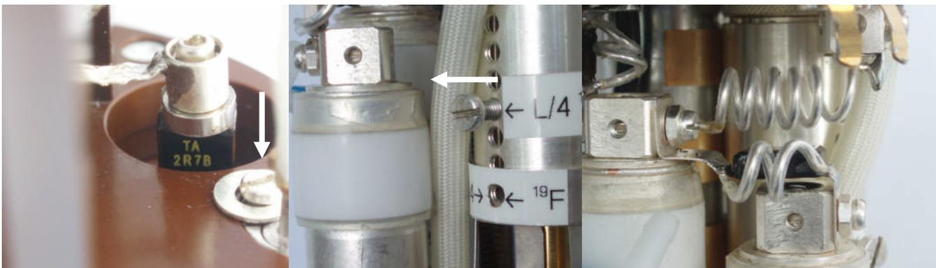
**Note:** The top of the transmission line is moveable. To use a serial C push down the transmission line to a mechanical stop. In the other case without serial C lift up the top of the transmission line as shown on the photo!
