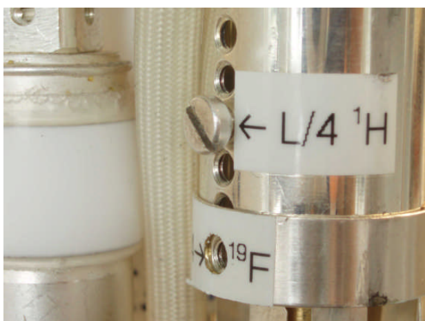
Figure 1 \lambda/4 -mode for ^1\text{H}
