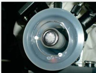
Fig. 3: The (thicker) coatings are clearly visible on the sample surface after it has dried. The incomplete coverage of the coating is likely due to the sample touching the window slightly when it was raised into the diffraction position.
