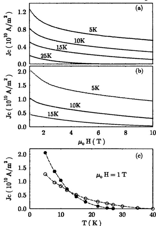
Figure 1:  $J_c$  vs  $\mu_0 H$  at the indicated temperatures: a) for Tl-2212 and b) for Bi-2212 single crystals. c)  $J_c$  vs  $T$  at the indicated fields: ● Tl-2212, ○ Bi-2212.
