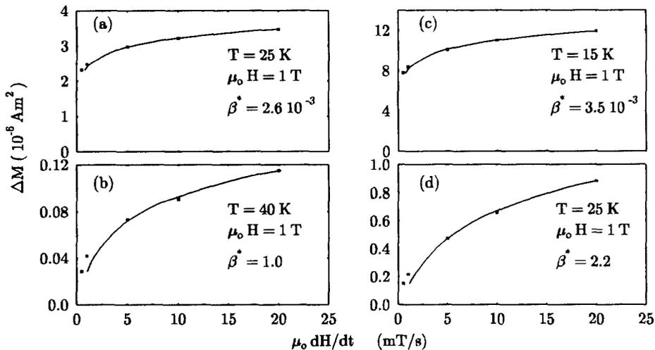
Figure 2: Magnetic hysteresis width ( $\Delta M$ ) versus magnetic sweep rate ( $\beta = \mu_0 dH/dt$ ) at the indicated temperatures, for Tl-2212 (a and b) and Bi-2212 (c and d). Lines represent a fit using eq.1.
