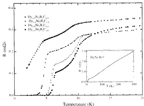
Fig. 4. Resistance vs. temperature curves for some  $\text{Dy}_x\text{Ni}_2\text{B}_2\text{C}_y$  compounds; the inset shows the resistance behaviour of the stoichiometric compound,  $\text{DyNi}_2\text{B}_2\text{C}$ , from 1.4–300 K.
