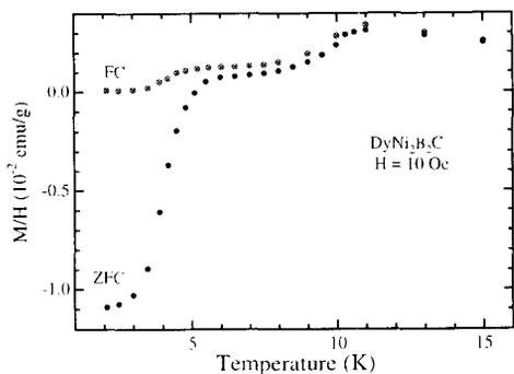
Fig. 3. Zero-field cooled (ZFC) and field-cooled (FC) magnetisation for  $\text{DyNi}_2\text{B}_2\text{C}$  measured in an applied field of 10 Oe, showing the superconducting transition at  $\sim 6$  K and the magnetic ordering at  $\sim 10.5$  K.
