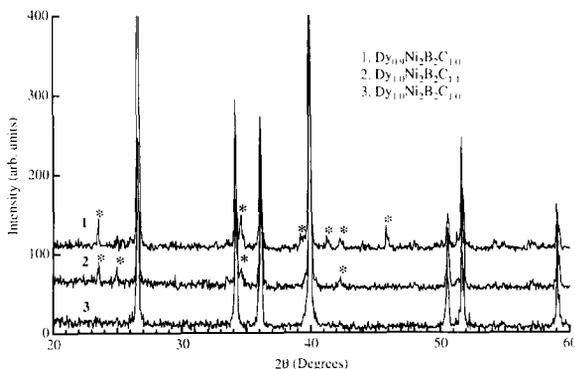
Fig. 1. X-ray powder diffraction patterns for a few of the  $\text{Dy}_x\text{Ni}_2\text{B}_2\text{C}_y$  compounds synthesized. The peaks corresponding to the impurity phases are marked with (\*).
