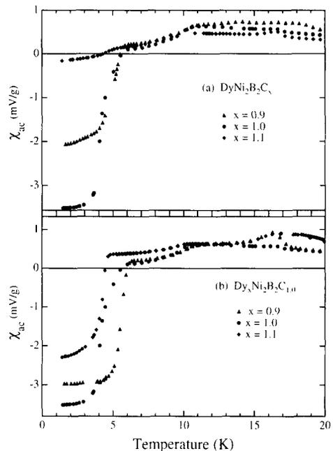
Fig. 2. Real part of the AC susceptibility ( $\chi_{AC}$ ) for the  $\text{Dy}_x\text{Ni}_2\text{B}_2\text{C}_y$  compounds, normalised to their masses, with (a) varying carbon content, (b) varying dysprosium content.
