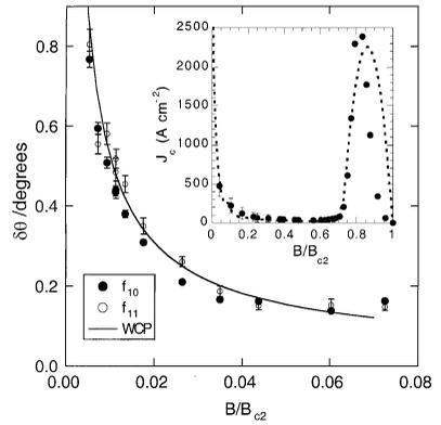
Fig. 2. The FWHM of the mosaic spread of the FLL ( $\delta\theta$ ) is shown as a function of applied field for diffraction from the lowest two order Bragg reflections. The line is a calculation for the WCP theory. The insert shows the critical current,  $J_c$ , for our sample at  $2.5 \text{ K}$ , deduced from magnetisation measurements. The dashed line is a calculation of  $J_c$  for the WCP parameter  $n\alpha^2/\xi^3 = 0.15$  consistent with the neutron scattering data.
