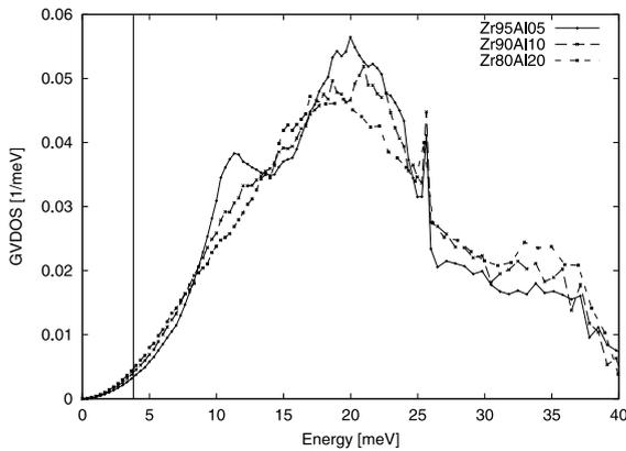
Fig. 2. GVDOS of  $Zr_{100-x}Al_x$  for  $x = 5, 10$  and  $20$ . The vertical line shows the energy region where the inelastic spectrum could not be separated from the foot of the huge elastic peak. The extremely sharp peak at about  $25.5$  meV (one time channel only!) is an artefact.
