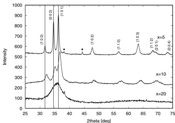
Fig. 1. X-ray diffraction pattern of  $Zr_{100-x}Al_x$ . The vertical lines makes clear the peak shifting, the points indicate the peaks of the Al sampleholder.
