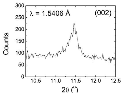
**Fig. 3** X-ray diffraction pattern showing the characteristic (002) peak of the AO/OO phase with the  $I4/mmm$  crystal structure as measured on a powdered piece of a  $Y_{0.15}Sr_{0.85}CoO_{3-\delta}$  single crystal.
