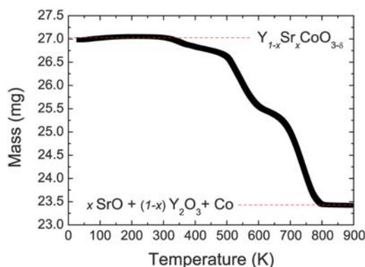
**Fig. 5** A typical TGA curve for the reduction of a powdered  $Y_{0.15}Sr_{0.85}CoO_{3-\delta}$  crystal in a 3%  $H_2/Ar$  atmosphere. This particular measurement was for the  $O_2$ -annealed  $Y_{0.15}Sr_{0.85}CoO_{3-\delta}$  crystal, but all the measurements for each of the crystals grown showed the same features.
