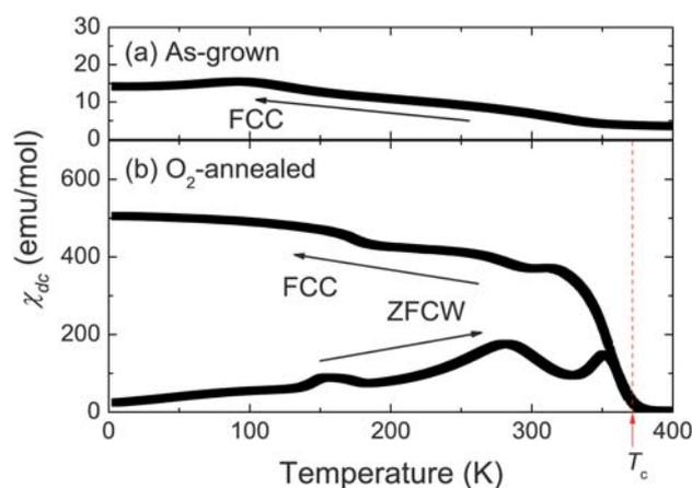
**Fig. 6** The temperature dependence of the zero-field cooled warming (ZFCW) and field-cooled cooling (FCC) dc magnetisation of a crystal of  $Y_{0.15}Sr_{0.85}CoO_{3-\delta}$ . Panel (a) shows the magnetisation for the as-grown crystal with a  $\delta$  value of 0.41 and panel (b) shows the magnetisation for the  $O_2$ -annealed crystal ( $H||c$ ) with a  $\delta$  value of 0.37. The measurements were made in an applied magnetic field  $\mu_0H = 0.1$  T.
