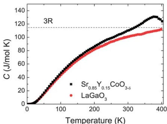
**Fig. 8** Temperature dependence of the specific heat of a single crystal of  $O_2$ -annealed  $Y_{0.15}Sr_{0.85}CoO_{3-\delta}$ .  $LaGaO_3$ , a non-magnetic perovskite, was also measured and is shown for comparison. The horizontal line indicates the value of  $3R$  per atom for YSCO.
