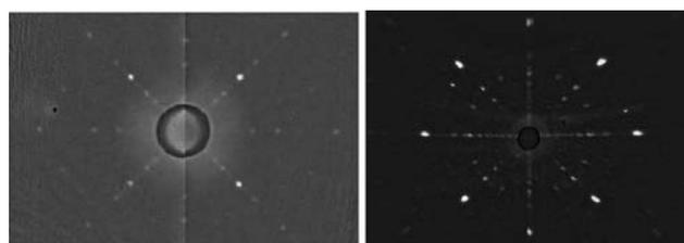
**Fig. 4** The left panel shows a typical X-ray Laue back-diffraction image obtained from a crystal of  $Y_{0.15}Sr_{0.85}CoO_{3-\delta}$  orientated along the  $c$  axis. The image was taken on a low voltage setting to avoid excessive cobalt fluorescence. The right panel shows a neutron Laue image along the same axis of the  $Y_{0.15}Sr_{0.85}CoO_{3-\delta}$  crystal.
