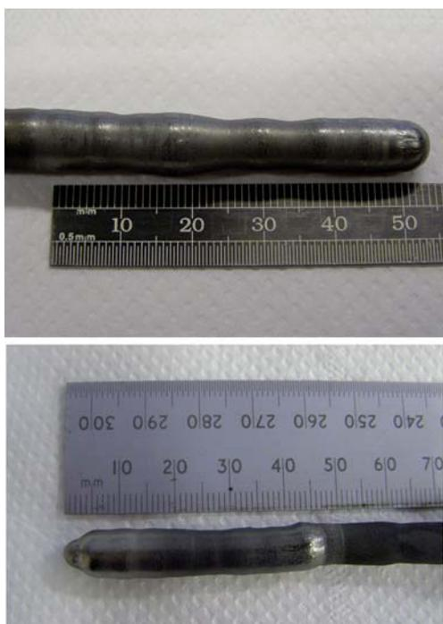
**Fig. 2** As-grown boules of  $Y_{0.15}Sr_{0.85}CoO_{3-\delta}$  (upper panel) and  $Y_{0.2}Sr_{0.8}CoO_{3-\delta}$  (lower panel) grown at speeds of 0.5–1 mm/h using the floating-zone method.
