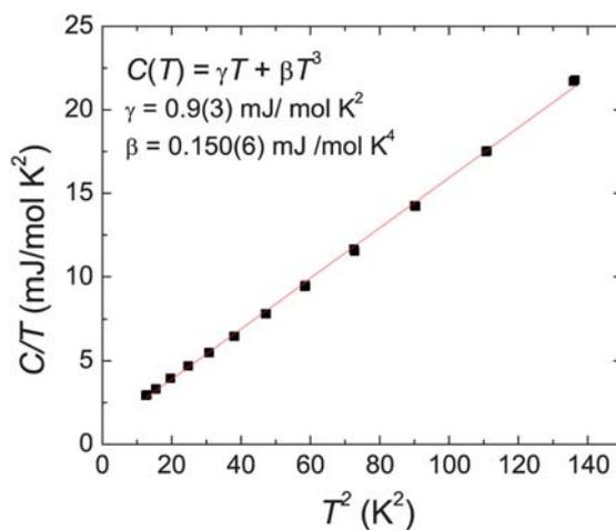
**Fig. 9**  $C/T$  vs  $T^2$  for the low temperature specific heat ( $2 < T < 12$  K) of a single crystal of  $O_2$ -annealed  $Y_{0.15}Sr_{0.85}CoO_{3-\delta}$ . The fit is to a model consisting of the electronic ( $\gamma T$ ) and the lattice ( $\beta T^3$ ) contributions to the specific heat, which is shown to be a good description of the low temperature data.
