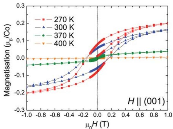
**Fig. 7** The field dependence of the dc magnetisation of an  $O_2$ -annealed crystal of  $Y_{0.15}Sr_{0.85}CoO_{3-\delta}$ . The sample was warmed above  $T_c$  between runs.
