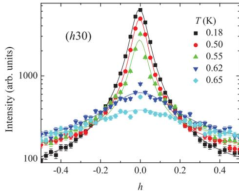
FIG. 5. (Color online) Temperature dependence of the scattering intensity of the (030) reflection from  $\text{SrHo}_2\text{O}_4$ . The data are fitted using the Lorentzian distribution and were collected using the D10 instrument at the ILL.
