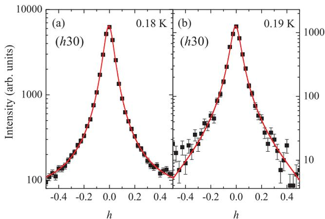
FIG. 12. (Color online) Comparison of the magnetic contribution to the scattering from SrHo<sub>2</sub>O<sub>4</sub> when scanning across the  $(030)$  peak in the (a) two-dimensional area detector configuration and (b) energy analyzer configuration. The peaks are fitted with a Lorentzian distribution, where the FWHMs are (a)  $(0.052 \pm 0.001) \text{ \AA}^{-1}$  and (b)  $(0.049 \pm 0.001) \text{ \AA}^{-1}$ .
