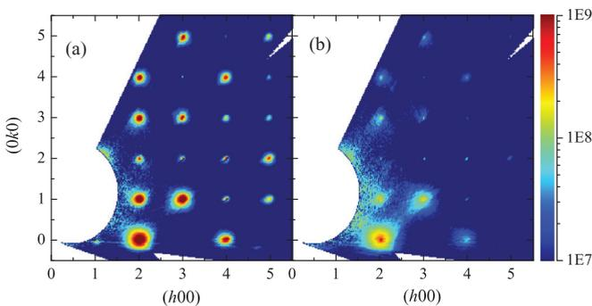
FIG. 2. (Color online) The magnetic contribution to the scattering from SrHo<sub>2</sub>O<sub>4</sub> in the (*hk*0) plane at (a) 0.055 K and (b) 0.7 K. The magnetic component was isolated by subtracting a 1-K background from the single-crystal neutron-diffraction data collected using WISH, ISIS.<sup>37</sup>
