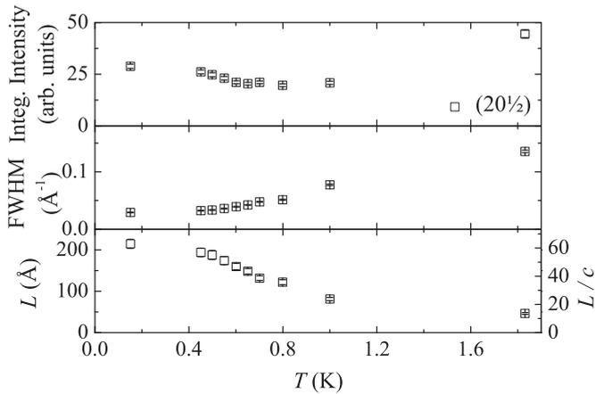
FIG. 11. Temperature dependence of the integrated intensity and the FWHM along  $l$  of the  $(20\frac{1}{2})$  reflection from SrHo<sub>2</sub>O<sub>4</sub>. The calculated correlation length  $L$  along the  $c$  axis is shown in the bottom panel, with the right-hand axis giving a conversion to how many unit cells the magnetic order is correlated to. The integrated intensity and the FWHM were extracted by fitting a Lorentzian distribution to data collected using the D10 instrument at the ILL.
