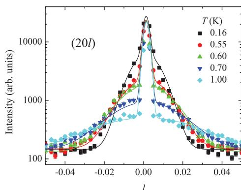
FIG. 6. (Color online) Temperature dependence of the scattering intensity of the (200) reflection from  $\text{SrHo}_2\text{O}_4$ . The data are fitted using two Gaussian components (one for nuclear and one for magnetic contributions) at all temperatures. The data were collected using the D10 instrument at the ILL.
