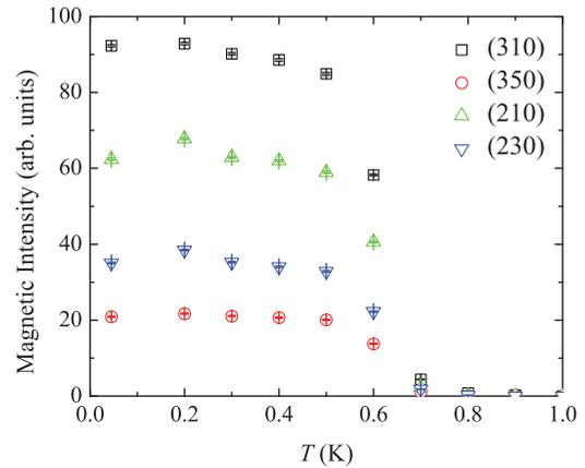
FIG. 3. (Color online) Temperature dependence of several diffuse peaks intensities in the (*hk*0) plane as a function of temperature. The magnetic intensity was isolated by subtracting a 1-K background from data collected using WISH, ISIS.
