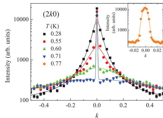
FIG. 4. (Color online) Temperature dependence of the scattering intensity of the (200) reflection from SrHo<sub>2</sub>O<sub>4</sub>. The data are fitted using Gaussian (nuclear) and Lorentzian (magnetic) components and were collected on the D10 instrument at the ILL. Inset: Data collected for the nuclear (200) peak at high temperature with high resolution and the fitted Gaussian distribution.
