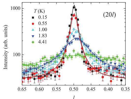
FIG. 10. (Color online) Temperature dependence of the integrated intensity of the diffuse magnetic scattering around  $(20\frac{1}{2})$ , measured using the D10 instrument at the ILL. The data have been fitted using a Lorentzian distribution.
