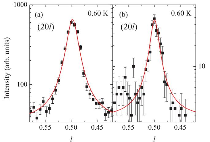
FIG. 13. (Color online) Comparison of the diffuse magnetic scattering when scanning along  $(20l)$  in the (a) two-dimensional area detector configuration and (b) energy analyzer configuration. When the data are fitted with a Lorentzian distribution, the FWHMs are (a)  $(0.039 \pm 0.002) \text{ \AA}^{-1}$  and (b)  $(0.029 \pm 0.003) \text{ \AA}^{-1}$ .
