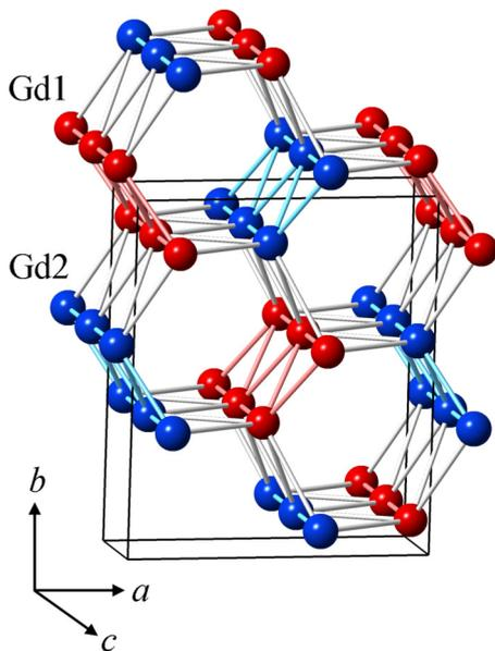
FIG. 1. (Color online) Positions of the magnetic ions in  $\text{SrGd}_2\text{O}_4$ , with the two crystallographically inequivalent sites of the rare-earth ions shown in different colors (red and blue). When viewed in the  $a$ - $b$  plane, honeycombs of the  $\text{Gd}^{3+}$  ions are visible. Zigzag chains running along the  $c$  axis connect the honeycomb layers and give rise to geometric frustration. The box indicates the dimensions of the crystallographic unit cell.
