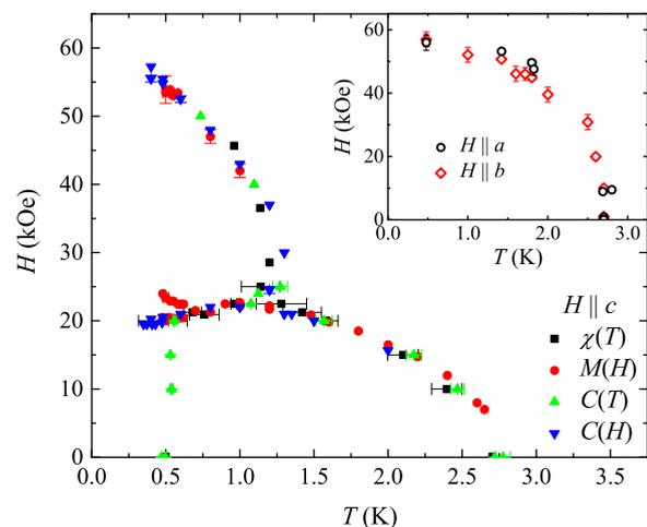
FIG. 9. (Color online) Magnetic  $H$ - $T$  phase diagram for  $\text{SrGd}_2\text{O}_4$  with the field applied along the  $c$  axis constructed from the susceptibility, magnetization, and specific heat curves. (Inset) Field dependence of the upper critical temperature,  $T_{N1}$ , as observed in magnetization  $M(H)$  and  $M(T)$  measurements for  $H \parallel a$  and  $H \parallel b$ . The methods used to obtain the phase boundaries are given in Ref. [41].
