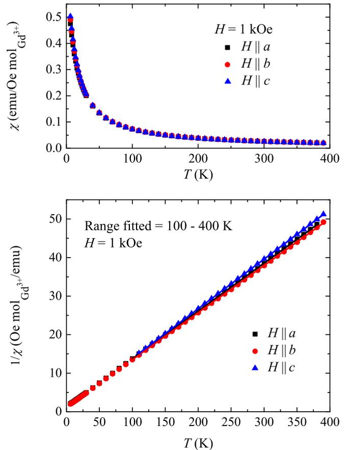
FIG. 2. (Color online) (Top) Magnetic susceptibility vs temperature in an applied field of 1 kOe in the temperature range of 6 to 400 K for the field applied along the three principal axes of a single-crystal sample of  $\text{SrGd}_2\text{O}_4$ . (Bottom) Reciprocal of the molar susceptibility vs temperature and the least-squares regression fits to the data (using the Curie-Weiss model).
