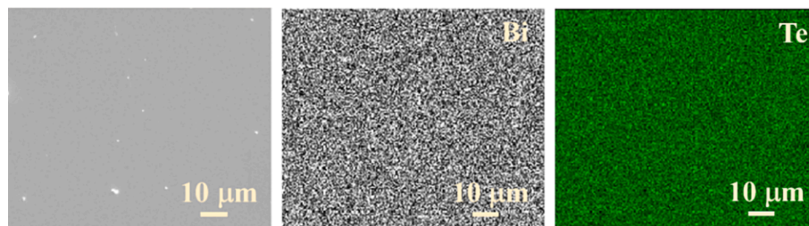
Fig. 3. Example of SEM image and EDS elements maps on \text{Bi}_2\text{Te}_3 crystals grown by procedure II + FZ. No impurities were detected in this case.
