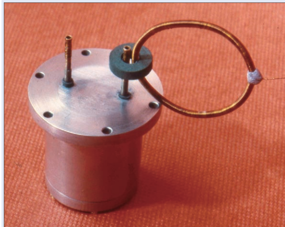
When a ring of \text{YBa}_2\text{Cu}_3\text{O}_{7-d} is subjected to deliberate electromagnetic interference, the magnetic flux jumps in and out of the ring in integer multiples of the flux quantum (top). In accordance with BCS theory, the value of this flux quantum was measured to be h/2e . The photograph (bottom) shows the apparatus used to measure the flux quantum – complete with Blu-Tack. (Adapted from C E Gough et al. 1987 Nature 326 855)
