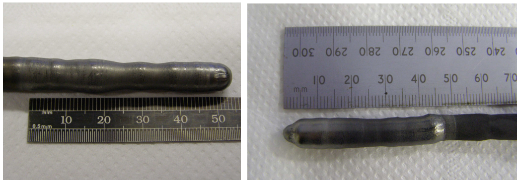
Figure 5.1: As-grown boules of Y 0.15 Sr 0.85 CoO 3-δ (left panel) and Y 0.2 Sr 0.8 CoO 3-δ (right panel) grown at speeds of 0.5-1 mm/hr using the floating-zone method.
