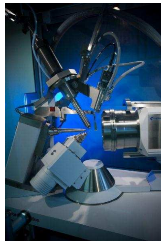
Figure 3.5: An Oxford Diffraction CCD single crystal diffractometer. The figure shows the sample on a four-circle goniometer, the cryo-jet, X-ray source, CCD and beam stop.
