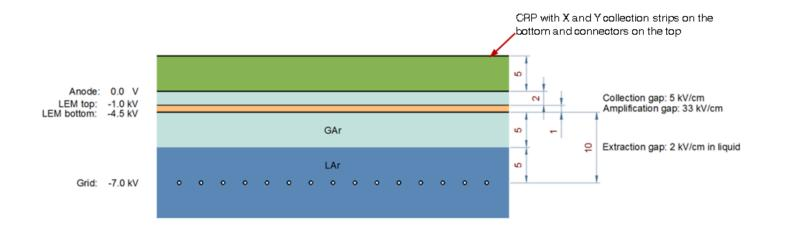
• 1 CRP = sandwich of 36 LEMs + 1920 RO channels. ProtoDUNE-SP: 4 CRPs
