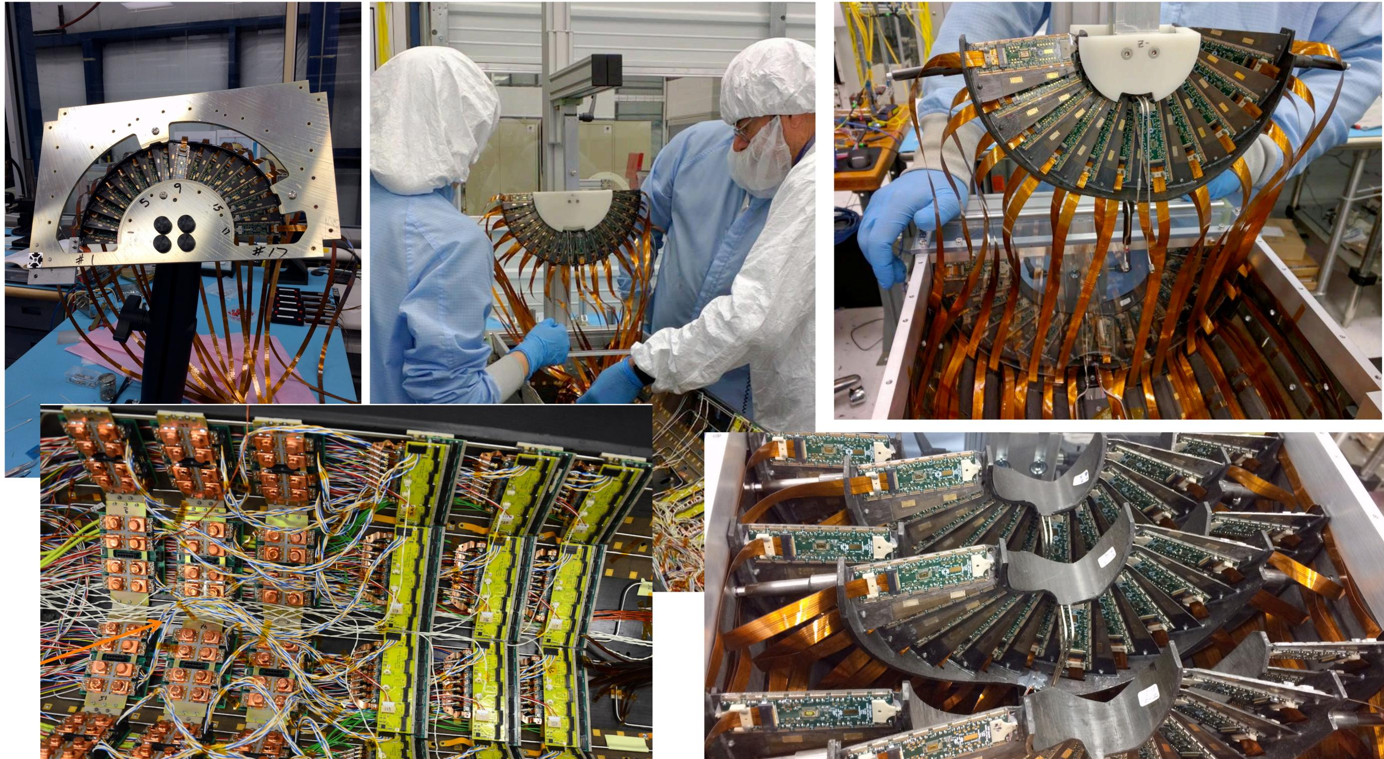
**All four half-cylinders tested with full DAQ readout chain at Fermilab**
