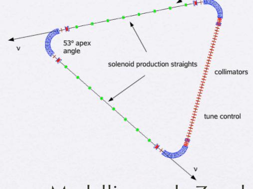
Modelling code Zgoubi being altered to allow study of storage rings, including bowtie and polarization effects.
