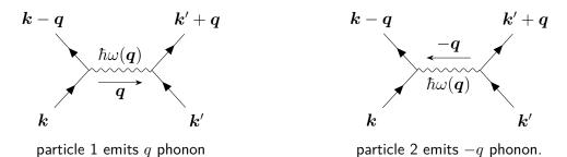
In both cases, electron 1 is scattered to k-q while electron 2 is scattered to k'+q. Energy conservation gives  $\epsilon(k)+\epsilon(k')=\epsilon(k-q)+\epsilon(k'+q)$ . According to second order perturbation theory, the amplitude for the scattering processes are
