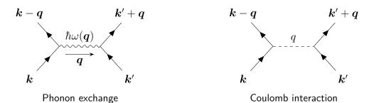
In the case of the phonon exchange, an electron with momentum k emits a phonon (lattice oscillation) with wavevector q and is scattered into a state with wavevector k-q. The phonon is absorbed by another electron with wavevector k'. This exchange is behind the phenomenon of superconductivity which we consider in the next chapter (see also Appendix C).
