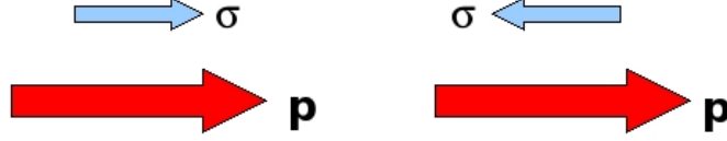
Figure 1: The two helicity states. On the left the spin vector is aligned in the direction of motions of the particle. This is a right-handed helicity state and has helicity +1. On the right the spin vector is antiparallel to the particle momentum. This is a left-handed helicity state with helicity -1.
