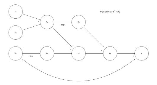
where the nodes  $x_4$  to  $x_8$  are the intermediate quantities that will have to be produced en route from the input values  $x_1$  to  $x_3$  to the final answer, f. The arrows run from *parent* nodes to *child* nodes. No child can be evaluated until all its parents have been evaluated.
