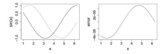
Note that the error appears to be of about the same magnitude as the finite difference interval  $\Delta$ . Perhaps we could reduce the error to around the machine precision by using a much smaller  $\Delta$ . Here is the equivalent of the previous plot, when
