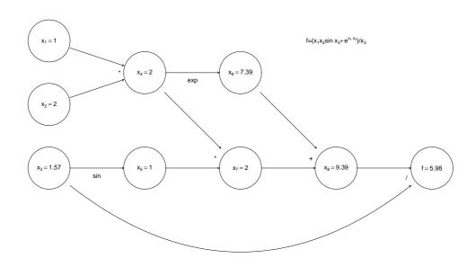
Now, forward mode AD carries derivatives forward through the graph, alongside values. e.g. the derivative of a node with respect to input variable,  $x_1$  is computed using
