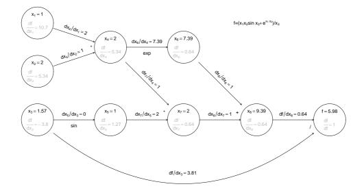
The derivatives in grey are those calculated on the reverse sweep. The point here is that there is only one derivative to be evaluated at each node, but in the end we know the derivative of f w.r.t. every input variable.
