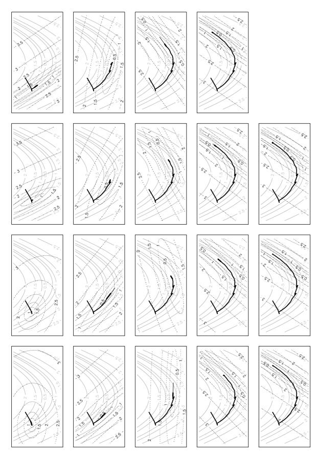
Notice how this quasi-Newton method has taken nearly twice as many steps as the Newton method, for the same problem, and shows a greater tendency to 'zig-zag'. However, it is still computationally cheaper than finite differencing for the Hessian, which would have required an extra 20 gradient evaluations, compared to quasi-Newton. Compared to steepest descent it's miraculous.
