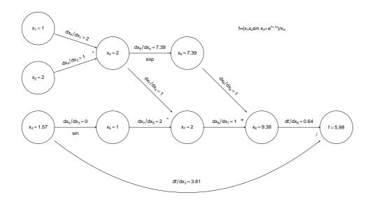
The *reverse* sweep then works backwards through the graph, evaluating the derivative of f w.r.t. each node, using the following
