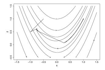
It took 14,845 steps to reach the minimum. This excruciatingly slow progress is typical of the steepest descent method. Another disadvantage of steepest descent is **scale dependence**: imagine linearly re-scaling so that the z axis in the above plot ran from -5 to 15, but the contours were unchanged. This would change all the steepest descent directions. By contrast, the methods considered next are scale invariant.
