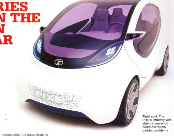
manoeuvring, the transmission's ability to control each rear wheel independently allows these wheels to rotate in opposing directions.
