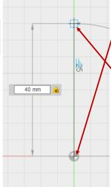
3) Click on the centre point then drag your mouse up. Type "40" to make your line 40mm long, then press the "Tab" button on your keyboard to lock the dimension in place. Left click once to position the line. Now drag the mouse to the right to draw another line. Make this Line 14mm in length. Press "Tab" to lock it. Then left click to position the line.
