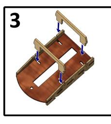
3. Slot the rib pieces into the chassis and the side panels. These ribs will give the vehicle strength and hold the parts in place firmly.
