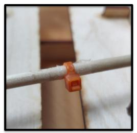
1. Wrap one small piece of tape around the middle of the axle. Tighten a cable tie over the tape. Trim the excess cable tie.
