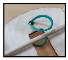
1. Poke an elastic band through the hole in the front of the chassis.
