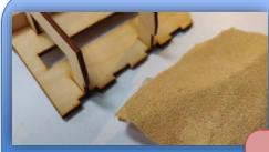
Use sandpaper to remove material from where it's hard to clip the parts together.
