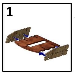
1. Slot the side panel pieces onto the chassis. These side panels have holes for your axles to fit through.
