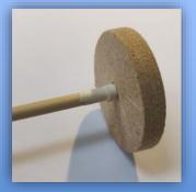
Put a single thickness of tape around the axle and gently twist the wheel over it.
