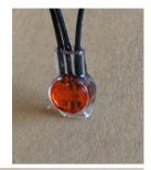
Wires are inserted into the crimp, take care to push them right to the back. Then use the crimp tool to squeeze the crimp closed. This pushes the metal crimp into the wires and makes a reliable connection.
