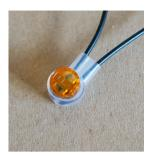
We'll use gel crimps, these are commonly used in telecom applications to make connections without the need to strip wires, solder or use breadboard.
