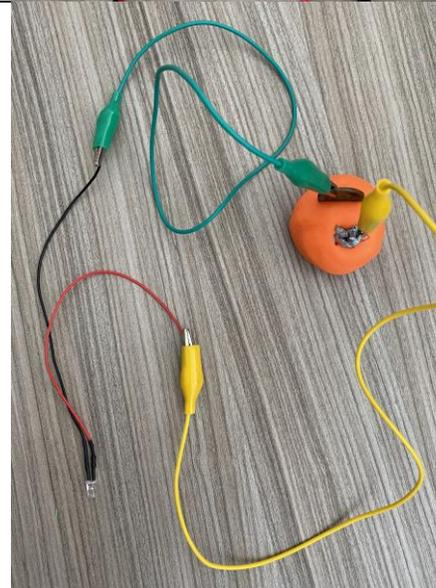
5. To make one big circuit with multiple battery cells make sure that one the LED connections is connected to the first coin and the other is connected to the last piece of zinc. Connect the battery cells in between from the zinc to the copper.
