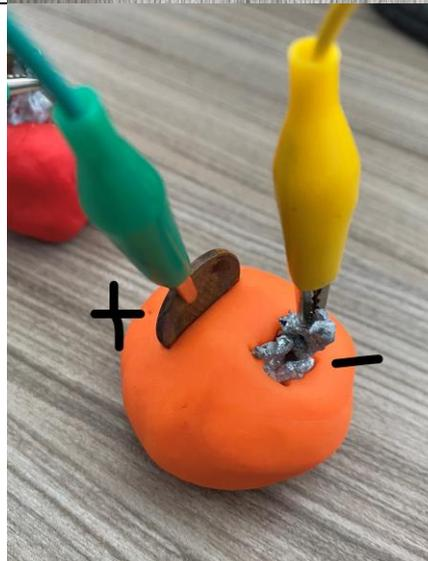
3. To test how much electricity is flowing through your playdough battery connect the crocodile clips to a voltmeter. For this example it was 0.758 V.
