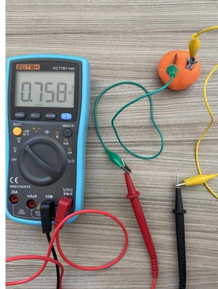
4. To connect it to the LED it is similar as for the battery. One LED needs around 2V to turn on so it didn't turn on with just one of the playdough battery cells. Try making a few more battery cells and then measuring the voltage to see how it changes.
