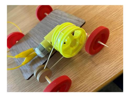
6. Using crocodile clips connect your motor with your batteries to produce a circuit
