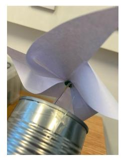
Carefully attach the paper windmill in the center, taped side down.  For safety reasons and to make your own solar updraft tower more attractive, add the pom pom ball or something similar to the top of the push pin.
