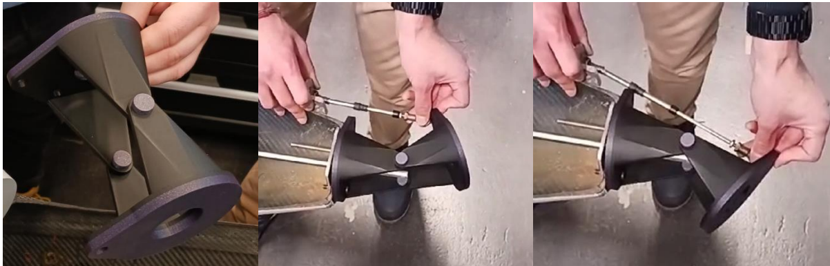
Figure 3 - How the push-pull cable (actuated by the pilots control stick) turns the propellor
