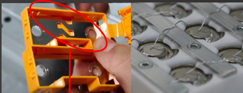
Multiple Fusible Links – Break short circuits (Kia/Tesla)
