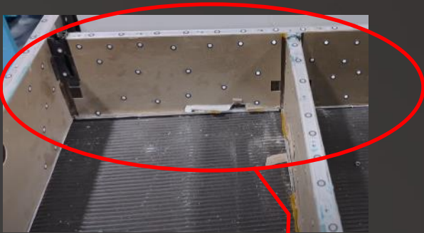
Tactical fireproof insulation on metallic parts – (BYD)
