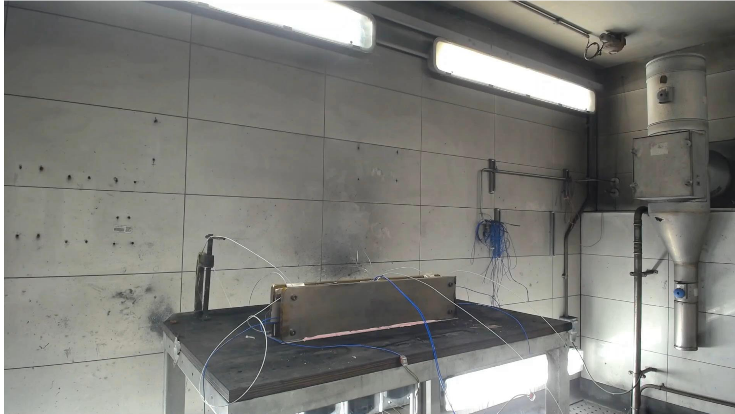
Progressive failure of 4 x 80 Ah pouch cells with fire barrier
