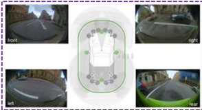
Figure 1. Four fisheye cameras mounted around the vehicle to provide complete 360-degree coverage.
