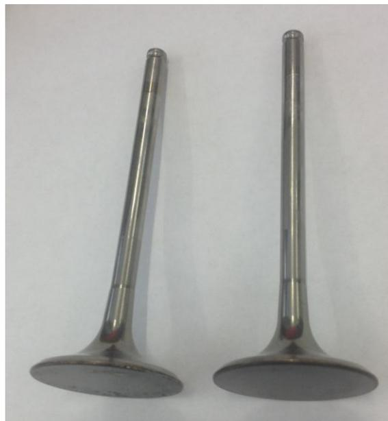
Figure 7: ALM intake valves post-test
