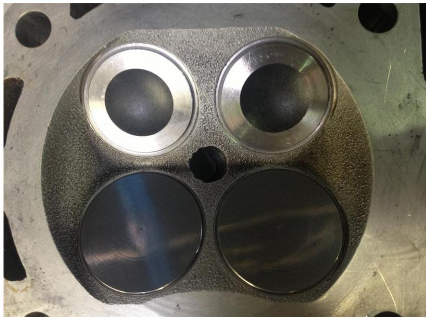
Figure 2: ALM intake valves installed alongside conventional exhaust valves in test engine cylinder head.
