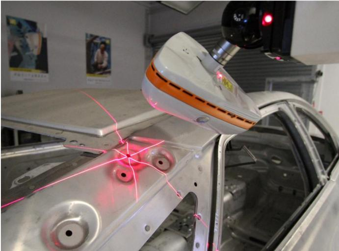
The WMG Product Evaluation Technologies Group, in collaboration with Nikon Metrology and Jaguar Land Rover, are investigating the optimisation of laser scanning technologies for production measurement systems in automotive applications.
