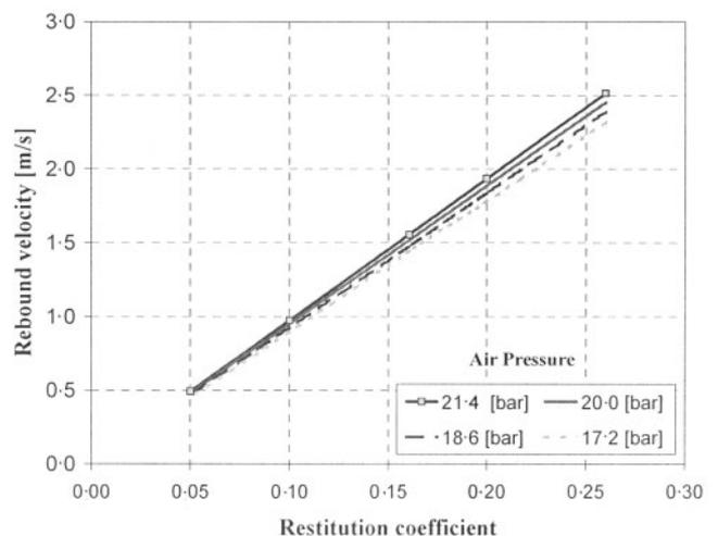
6 Variation of the piston rebound velocity versus restitution coefficient
