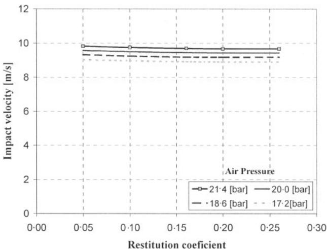
5 Piston impact velocity versus restitution coefficient
