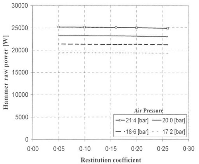
4 Hammer raw power versus restitution coefficient
