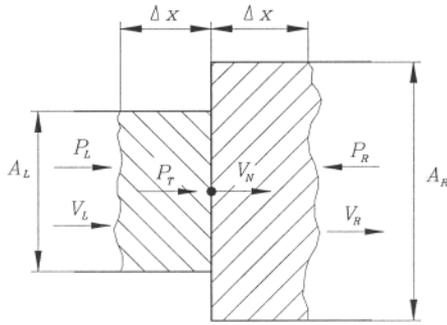
**B2 Linear momentum principle applied to a node between times  $t$  and  $t^+$**
