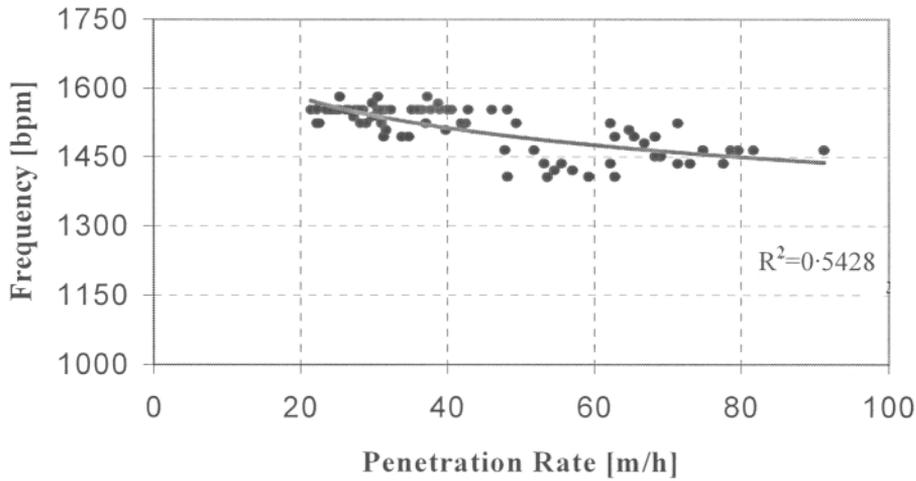
**13 Correlation between frequency and penetration rate (bpm, blows per minute)**
