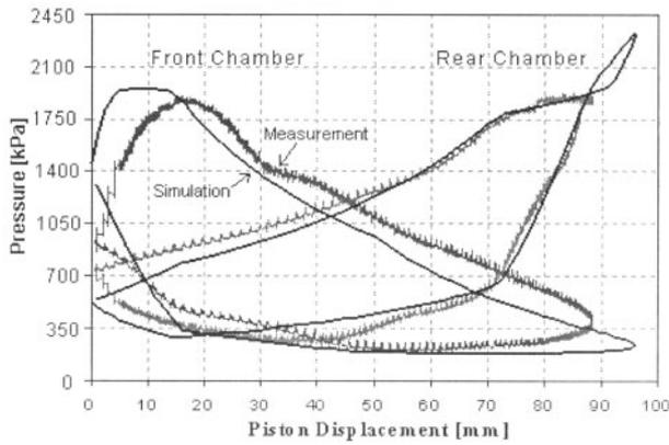
3 Actual and predicted front and rear chamber pressure versus piston displacement diagrams
