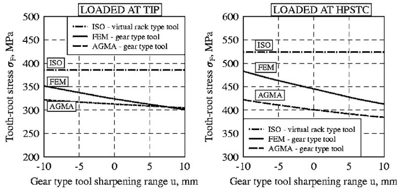
Fig. 20 Influence of the range of sharpening of gear tool (parameter  $u$ ) on tooth-root stress  $\sigma_F$  according to the ISO, AGMA, and FEM: for load applied at the tip (left) and for load applied at the HPSTC (right); main parameters of the gear tool (generating tool) and the gear in section 0-0 are the same as in Fig. 11; magnitude of load is the same as in Fig. 18
