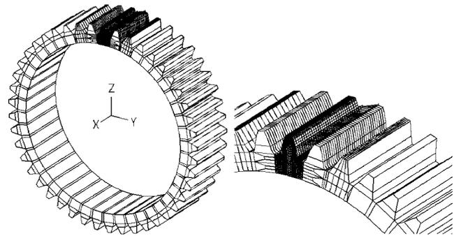
Fig. 3 The FEM model of a representative gear ( $z=45$ ,  $m_n=2.75$  mm,  $\alpha_n=20$  deg,  $b=32$  mm) made of 3D 20-node isoparametric and eight-node brick finite elements; all degrees of freedom on the internal cylinder of gear disk fixed; load uniformly distributed along the line of contact at the HPSTC; model of the whole gear (left); enlarged view of the loaded tooth (right)
