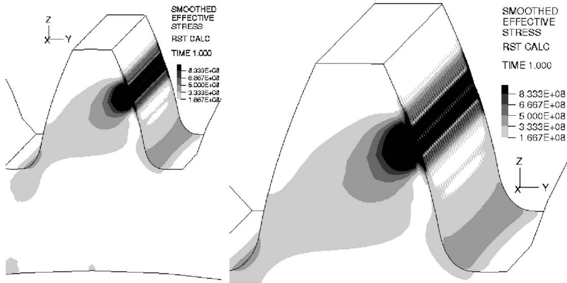
Fig. 5 Distribution of the effective stress in the loaded tooth of the gear shown in Fig. 3
