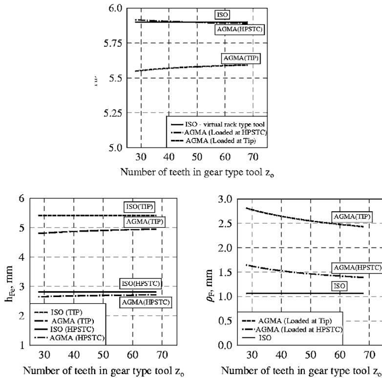
**Fig. 15** Influence of the number of teeth  $z_0$  of the gear tool on parameters of the critical section:  $s_{Fn}$ ,  $h_{Fe}$ ,  $\rho_F$  according to the ISO, AGMA for load applied at the tip (Tip) and at the HPSTC; main parameters of the gear tool (generating tool) and gear are the same as in Fig. 11
