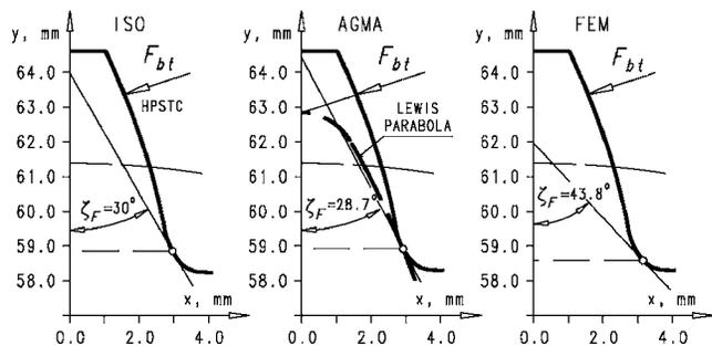
**Fig. 26** Comparison of locations of the critical section and the angle between tangent to fillet and tooth centerline computed according to the ISO (left) and AGMA (middle) standards as well as according to the precise finite element analysis (right) of the gears with the same tooth profiles; magnitude of load is the same as in Fig. 18
