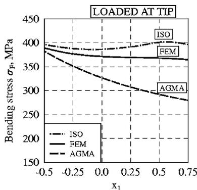
Fig. 22 Influence of the addendum modification coefficient  $x_1$  on tooth-root stress  $\sigma_F$  according to the ISO, AGMA, and FEM: for load applied at the tip; main parameters of the gear:  $m_n=2.75$ ,  $\alpha_n=20$  deg,  $\beta_1=0$  deg; main parameter of the rack (generating tool):  $\rho_{IP}=0.18m_n$ ; magnitude of load is the same as in Fig. 18
