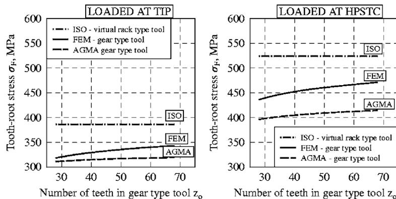
**Fig. 19 Influence of the number of teeth  $z_0$  of the gear tool on tooth-root stress  $\sigma_F$  according to the ISO standard, AGMA standard, and FEM: for load applied at the tip (left) and for load applied at the HPSTC (right); main parameters of the gear tool (generating tool) and gear are the same as in Fig. 11; magnitude of load is the same as in Fig. 18**
