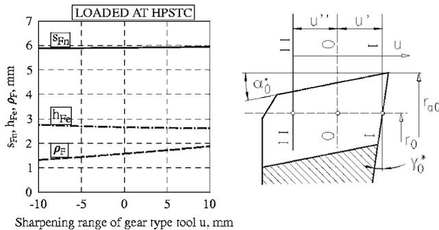
**Fig. 16** Influence of the range of sharpening of gear tool (parameter  $u$ ) on parameters of the critical section:  $s_{Fn}$ ,  $h_{Fe}$ ,  $\rho_F$  according to the AGMA standard for load applied at the HPSTC (left), the range of sharpening of gear tool (right); main parameters of the gear tool (generating tool), and the gear in section 0-0 are the same as in Fig. 11
