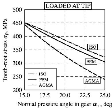
Fig. 21 Influence of the normal pressure angle  $\alpha_n$  on tooth-root stress  $\sigma_F$  according to the ISO, AGMA, and FEM: for load applied at the tip; main parameters of the gear:  $m_n=2.75$ ,  $z_1=45$ ,  $s_1=4.265$ ,  $\beta_1=0$  deg; main parameters of the rack (generating tool):  $s_0=4.320$ ,  $\rho_{IP}=0.18m_n$ ; magnitude of load is the same as in Fig. 18
