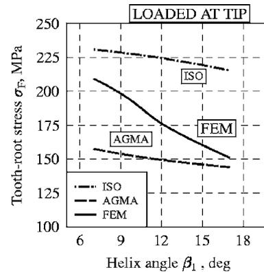
Fig. 23 Influence of the helix angle  $\beta_1$  on tooth-root stress  $\sigma_F$  according to the ISO, AGMA, and FEM for load applied at the tip; main parameters of the gear:  $m_n=5.0$ ,  $z_1=24$ ,  $\alpha_n=20$  deg, magnitude of distributed load passing through the tip corner of helical tooth flank  $F_{bn}/b=274$  N/mm
