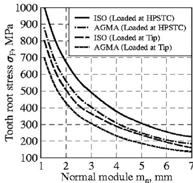
**Fig. 25** Influence of the normal module  $m_n$  on tooth-root stress  $\sigma_r$  according to the ISO and AGMA for load applied at the tip (Tip) and at the HPSTC; main parameters of the generating rack and gear are the same as in Fig. 12; magnitude of load is the same as in Fig. 18
