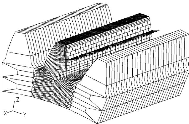
Fig. 2 The FEM model of a representative gear ( $z=45$ ,  $m_n=2.75$  mm,  $\alpha_n=20$  deg,  $b=32$  mm): segment of three-tooth made of 3D isoparametric 20-node brick finite elements; boundary conditions as in Fig. 1; load uniformly distributed along the line of contact at the HPSTC
