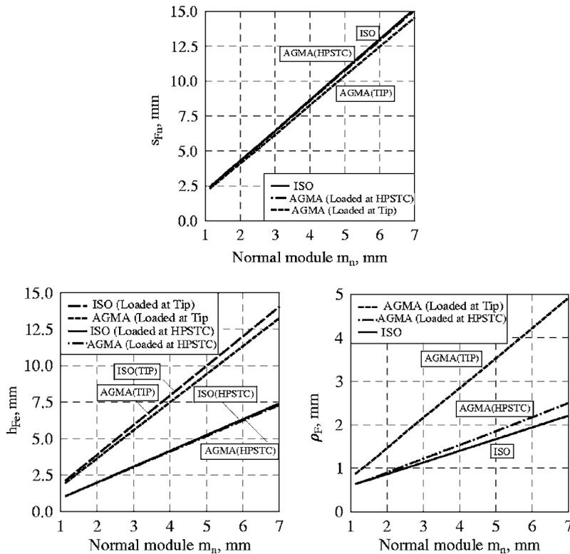
**Fig. 17 Influence of the normal module  $m_n$  on parameters of the critical section:  $s_{Fn}$ ,  $h_{Fe}$ ,  $\rho_F$  according to the ISO and AGMA standards for load applied at the tip (Tip), and at the HPSTC; main parameters of the rack (generating tool) and gear are the same as in Fig. 12**
