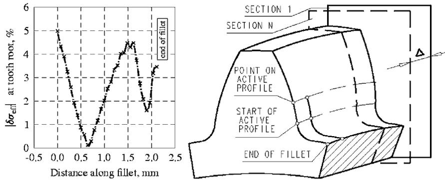
**Fig. 7 Absolute values of obtained differences in the effective stresses along fillet  $\delta\sigma_{\text{eff}}$  computed according to Eq. (1) for the 2D plane stress model with three teeth and for the model of the whole gear built of 3D 20-node isoparametric and eight-node brick finite elements in sections associated with  $\Delta=2$  mm (left); explanation of the sections and the lines where the effective stresses are compared (right)**
