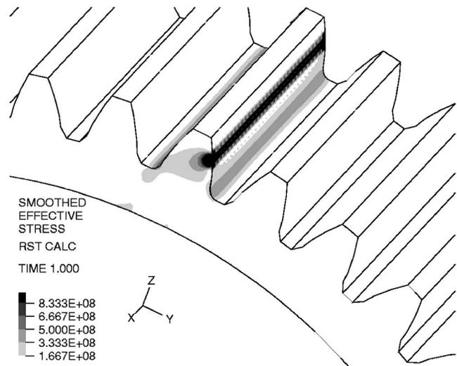
Fig. 4 Distribution of effective stress in the loaded part of the whole gear shown in Fig. 3
