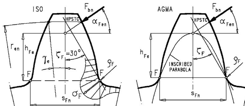
**Fig. 9 Determination of the critical section location, angle  $\zeta_F$  and parameters of the critical section  $s_{Fn}$ ,  $h_{Fe}$ , and  $\rho_F$ ; according to the ISO and the AGMA standards (for comparison see Table 7 in the Appendix)**
