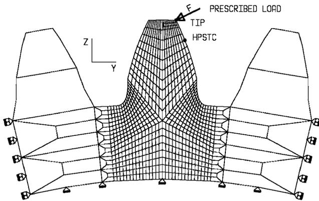
Fig. 1 The finite element model of a segment of a gear and two load cases: prescribed force applied at the tip and prescribed force applied at the highest point of single tooth contact (HPSTC)
