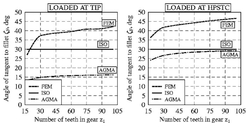
**Fig. 10 Influence of the number of gear teeth on the angle  $\zeta_F$  between tooth centerline and tangent to fillet at the critical point  $F$  according to the ISO standard, AGMA standard, and FEM: load applied at the tip (left), load applied at the HPSTC (right); main parameters of the gear:  $m_n=2.75$ ,  $\alpha_n=20$  deg,  $s_1=4.265$ ,  $\beta_1=0$  deg, main parameters of the rack:  $\alpha_0=20$  deg,  $s_0=4.320$ ,  $h_{IP}=1.22m_n$ ,  $\rho_{IP}=0.18m_n$**
