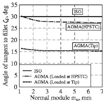
**Fig. 12 Influence of the normal module  $m_n$  on the angle  $\zeta_F$  between tooth centerline and tangent to fillet at the critical point  $F$  according to the ISO standard, AGMA standard for load applied at the tip (Tip), and at the HPSTC; main parameters of the gear:  $z_1 = 45$ ,  $\alpha_n = 20$  deg,  $\beta_1 = 0$  deg; main parameters of the rack:  $\alpha_0 = 20$  deg,  $h_{fP} = 1.25m_n$ ,  $\rho_{fP} = 0.5$**
