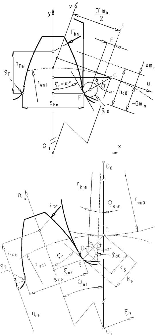
**Fig. 13 Determination of parameters of the critical section:  $s_{Fn}$ ,  $h_{Fe}$ , and  $\rho_F$ , according to the ISO standard (top) and according to the AGMA standard (bottom)**
