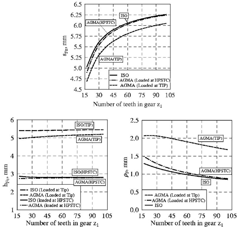
**Fig. 14 Influence of the number of gear teeth  $z_1$  on parameters of the critical section:  $s_{Fn}$ ,  $h_{Fe}$ ,  $\rho_F$  according to the ISO, AGMA for load applied at the tip (Tip), and at the HPSTC; main parameters of the rack (generating tool) and gear are the same as in Fig. 10**
