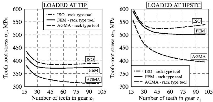
**Fig. 18 Influence of the number of gear teeth  $z_1$  on tooth-root stress  $\sigma_F$  according to the ISO standard, AGMA standard, and FEM: for load applied at the tip  $F_{bn}/b=250$  N/mm (left) and for load applied at the HPSTC  $F_{bn}/b=500$  N/mm (right); main parameters of the rack (generating tool) and gear are the same as in Fig. 10**
