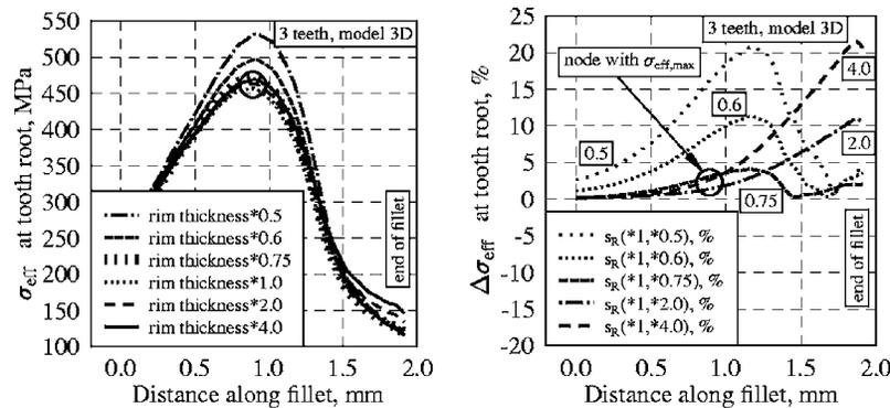
**Fig. 8 Comparative analysis of the effective stress distribution at tooth root for three magnitudes of rim thickness of gear (left); absolute values of the relative differences in the effective stresses along fillet  $\Delta\sigma_{\text{eff}}(1, i)$  computed according to Eq. (2) for the model of three-teeth segment of gear built of 3D 20-node isoparametric, for load applied at the HPSTC  $F_{bn}/b=500$  N/mm (right)**
