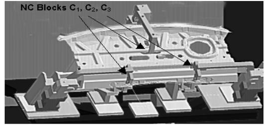
Figure 3: Part located on fixture and clamped with NC blocks.
