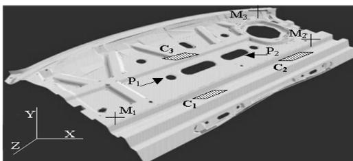
Figure 2: Locator and sensor distribution on part
