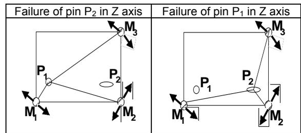
Figure 4: Geometric interpretations of failures in Z axis
