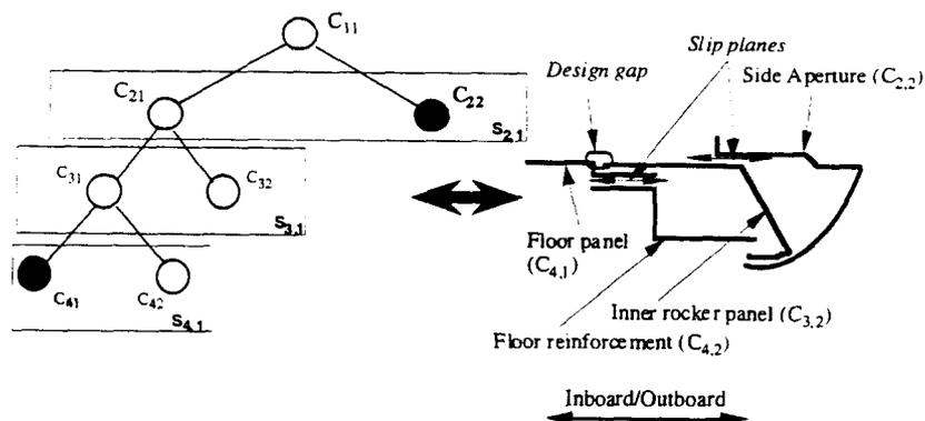
Fig. 10 Design 1: aperture-underbody
