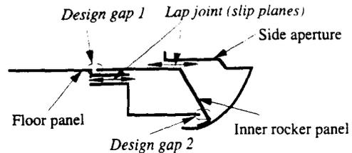
Fig. 3 Design 1: an example of lap joints and a design gap
