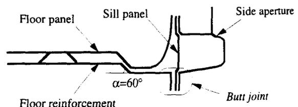
Fig. 4 Design 2: an example of butt joints
