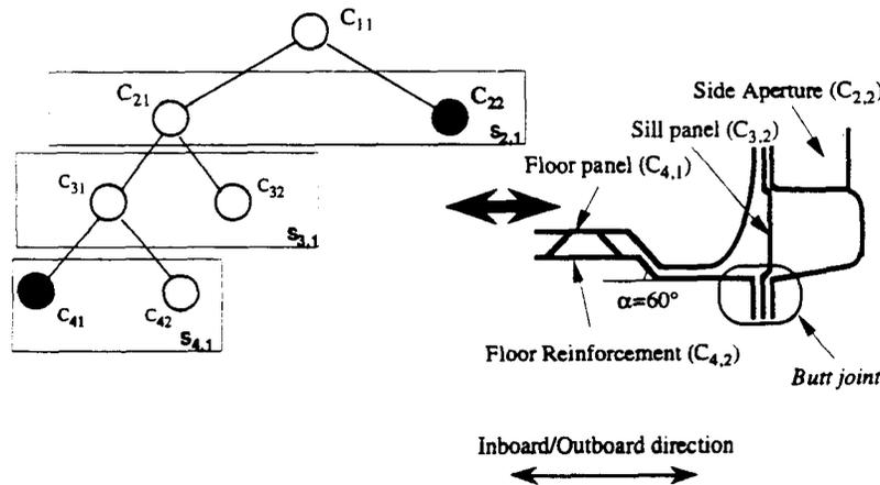
Fig. 11 Design 2: aperture-underbody
