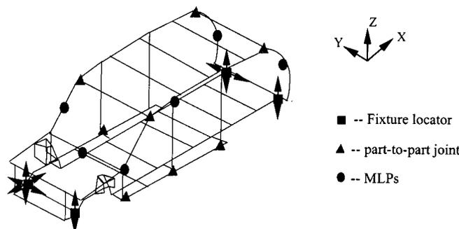
**Fig. 3** The beam structure of an automotive body
