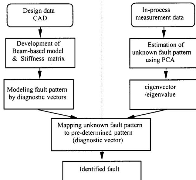
Fig. 1 The structure of the diagnostic methodology
