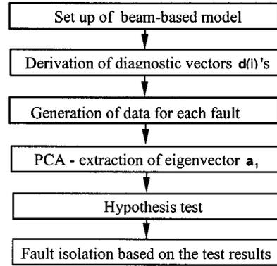
Fig. 4 The procedure for the conducted simulations
