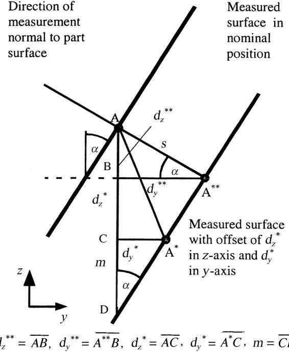
**Fig. 6.** Feature 2 level: geometrical relations for feature-based measurement error.
