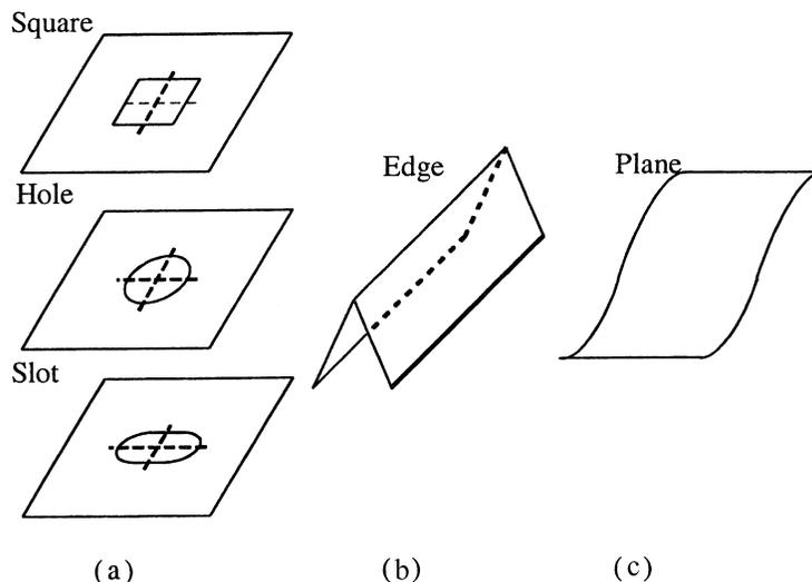
**Fig. 5.** A schematic diagram of the three selected measurement features: (a) square/hole/slot; (b) edge; and (c) plane.
