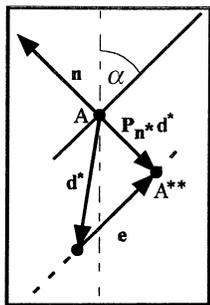
Fig. 8. Feature 3 level: geometric relations for feature-based measurement error.  $\mathbf{n}$ —unit measurement vector (perpendicular to the measured surface);  $\mathbf{d}^*$ —part displacement vector; and  $\mathbf{e}$ —feature-based measurement error.
