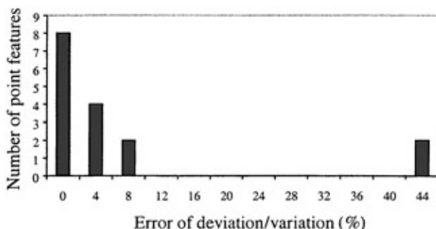
**Fig. 15.** Industrial case study 1: feature-based measurement error for automotive body measurement points (point features are level 3 features).
