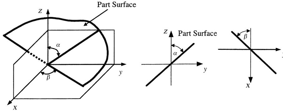
Fig. 7. Definition of angles for feature on measurement object.
