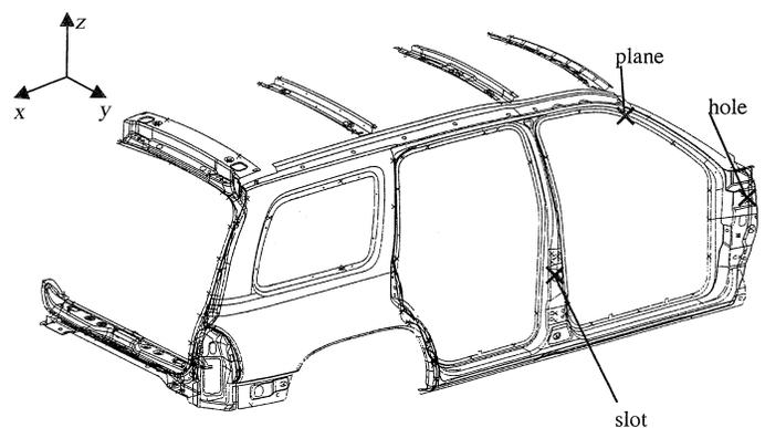
**Fig. 17.** Industrial case study 2: the feature-based measurement error for truck cab measurement point (point feature-level 3). Point A—measurement point marked as “plane” (level 3); and Point T—measurement point marked as “hole” (level 1) used for the compensation of the point A deviation in the z direction.
