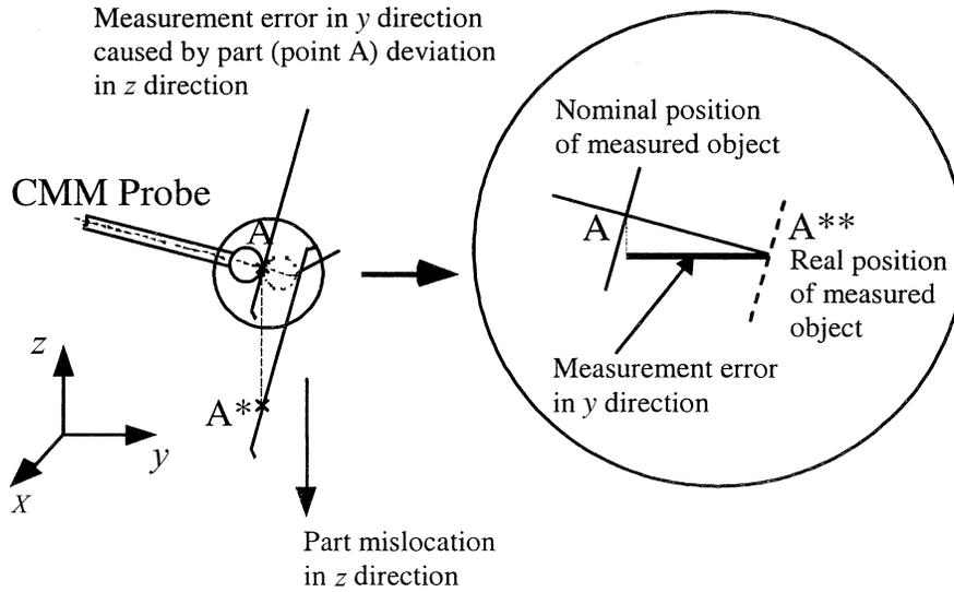
**Fig. 4.** A schematic diagram of the error in the  $y$  direction caused by a part mislocation in the  $z$  direction.  $A$ —nominal position of the measurement point;  $A^*$ —mislocated position of the measurement point caused by part mislocation in  $z$  direction; and  $A^{**}$ —point measured.
