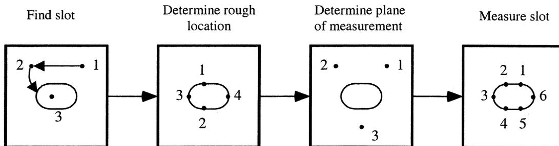
**Fig. 3.** An illustration of the use of the hole/slot feature algorithm.
