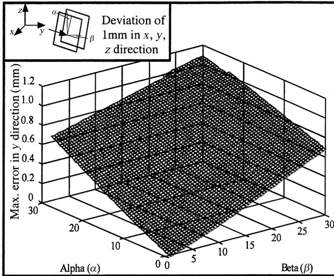
Fig. 12. Feature-based measurement error for simultaneous part deviation in the  $x$ ,  $y$  and  $z$  axes and  $\alpha$ ,  $\beta = (0, 30^\circ)$ .
