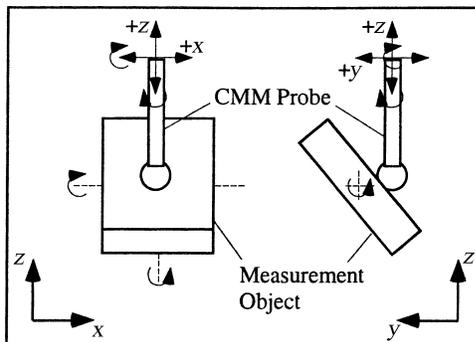
Fig. 13. Experimental setup.
