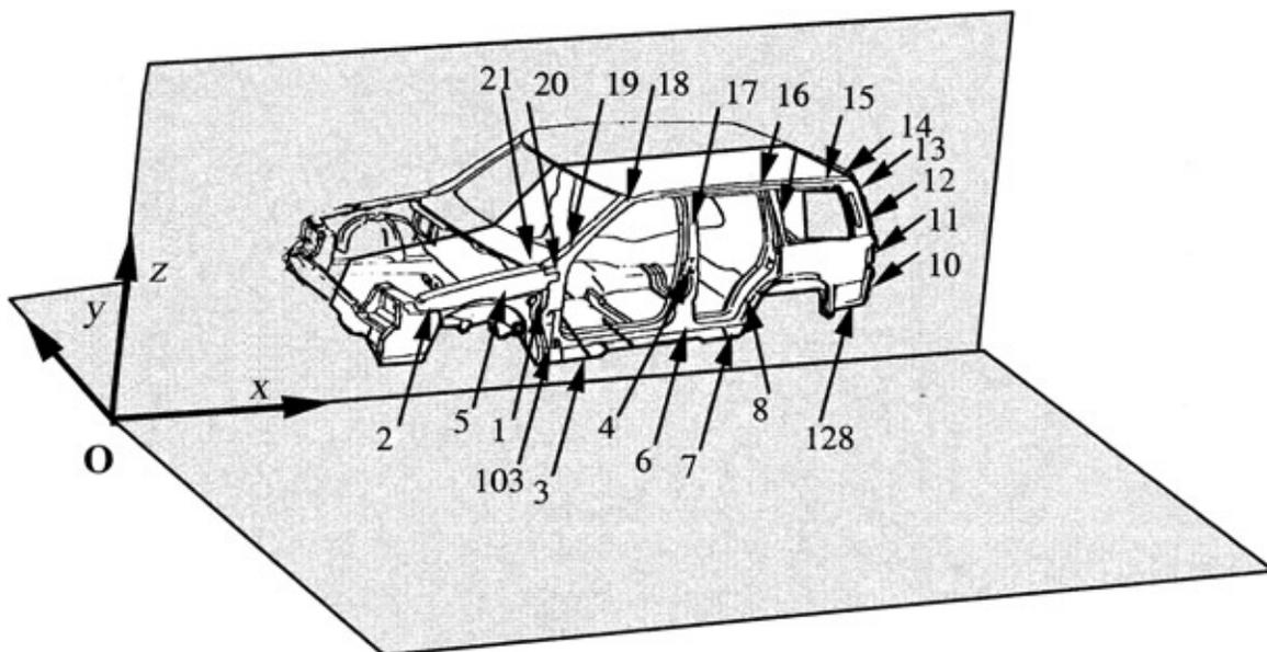
Fig. 1. The body coordinate system with an example of measurement point locations.
