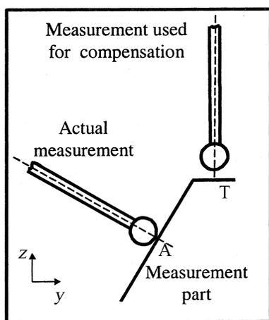
**Fig. 16.** An example of the relationships between a pair of measurement points [A, T]. Point A—actual measurement; Point T—measurement point used for compensation of the point A deviation in the z direction.
