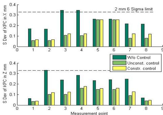
FIGURE 6. STANDARD DEVIATIONS OF THE MEASUREMENTS POINTS (KPCs).
