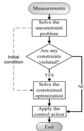
FIGURE 4. PROCEDURE TO DETERMINE THE CONTROL ACTION.
