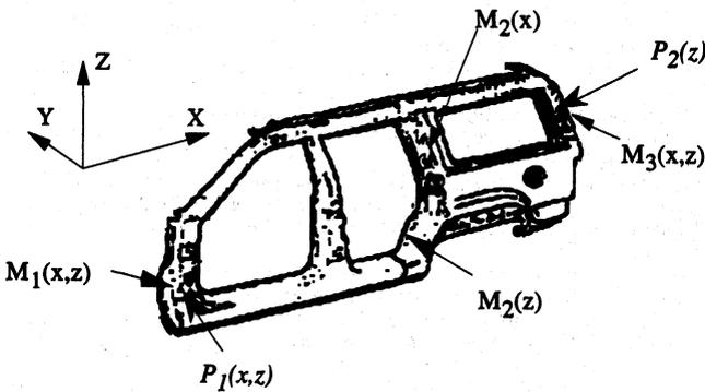
Fig. 8 Left handed aperture part with marked sensors and locating pins
