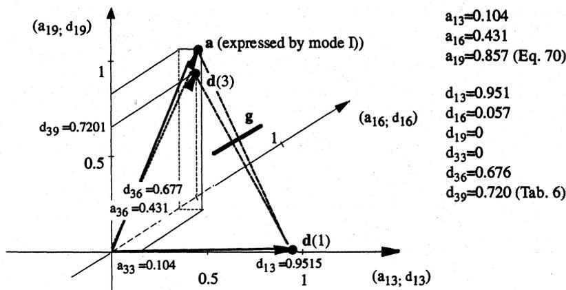
Fig. 10 Graphical representation of the fault mapping
