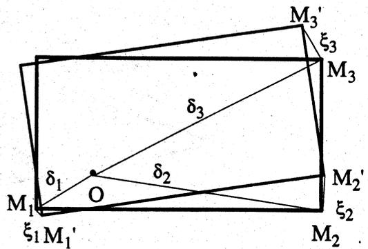
Fig. 3 Geometrical relations during rotation of the rigid part
