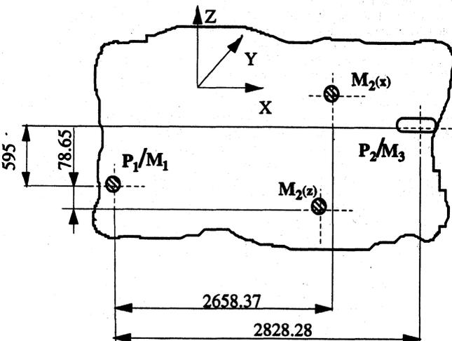
Fig. 9 Sensor location and the geometry of the fixture used in the Framing station
