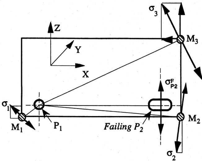
Fig. 4 Geometrical interpretation of the failing locator  $P_2$
