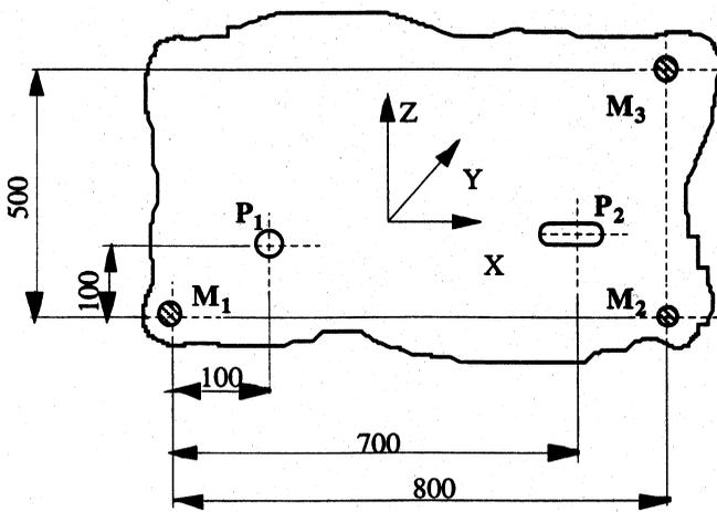
Fig. 6 The geometry of the fixture used for simulations
