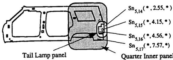
Fig. 14 Case study II-LH-APT scheme with marked elements of CSS set
