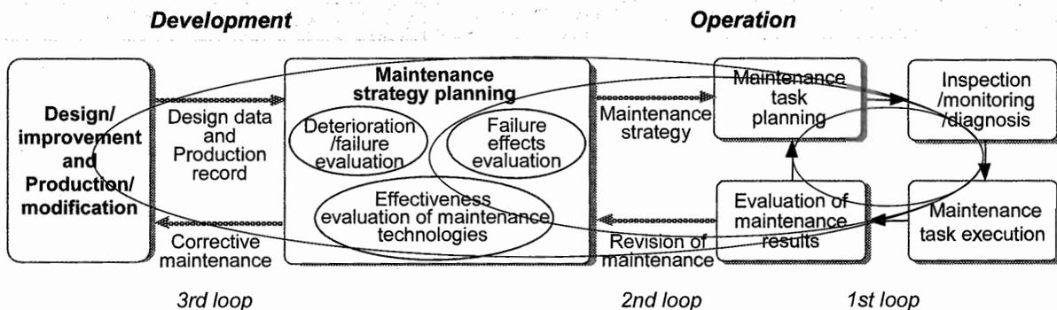
Figure 3: Framework for life cycle maintenance.
