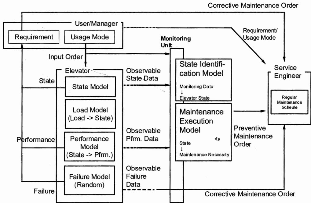
Figure 11: Simulation model for evaluating elevator maintenance strategies.
