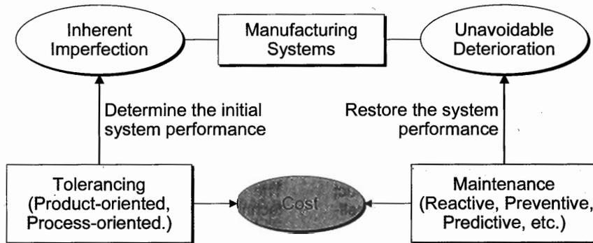
Figure 12: Integration of tolerance design and maintenance.
