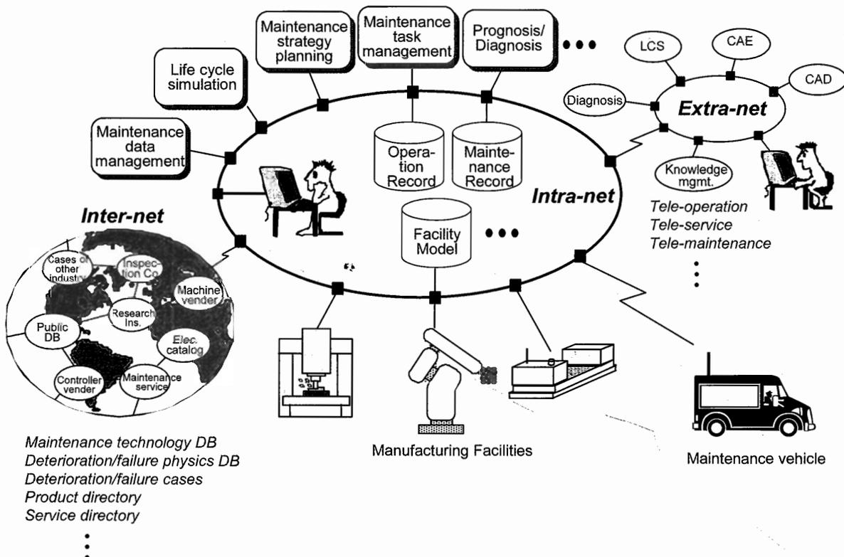
Figure 14: Concept of a web-based maintenance system.
