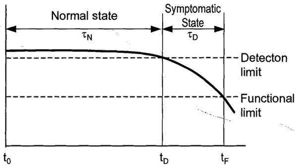
Figure 6: Progressive pattern of deterioration or functional degradation.
