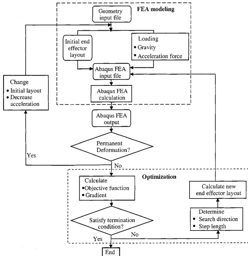
Fig. 5 The end effector layout design procedure
