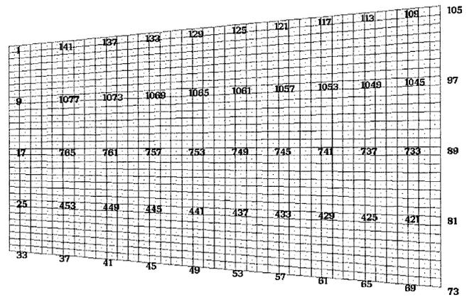
Fig. 10 FEA mesh and the critical points for the fender blank
