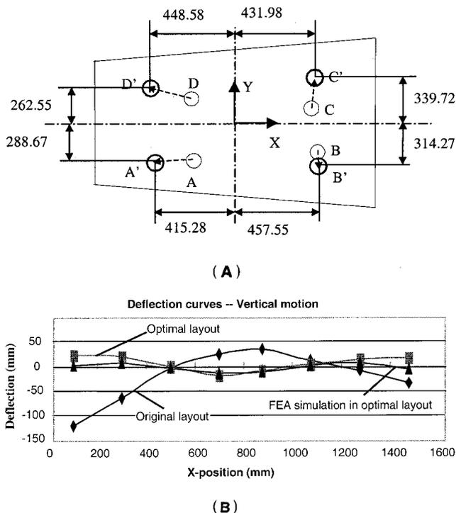
Fig. 13 Results of the FEA optimization and the test for the fender blank (a) The original and the optimal cup layout (b) Part deflection
