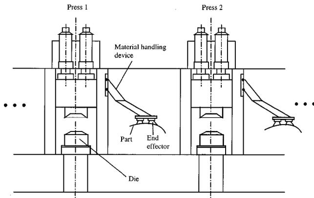
**Fig. 1** An example of a material handling system in a stamping line
