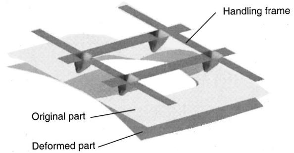
Fig. 7 Part deformation simulation
