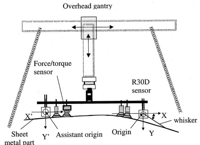
Fig. 11 The measurement setup
