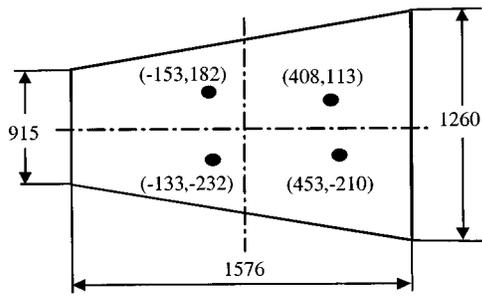
Fig. 9 Dimensions and the initial end effector layout for the fender blank
