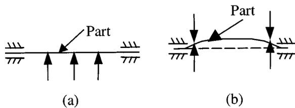
Fig. 4 Impact of the locating layout in the primary datum plane on the rigidity in the other two planes
