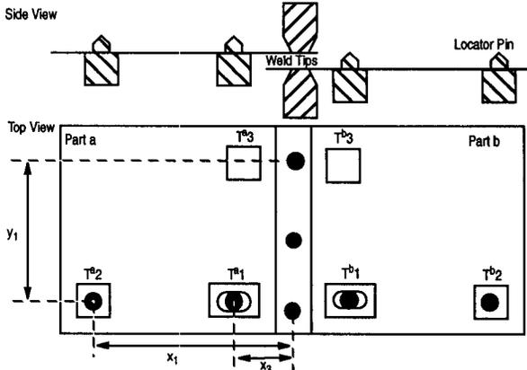
Part *a* and *b* are located based on a 3-2-1 scheme. The *z* direction is set by joints (welds), position of fixture locators and parts geometry. The lap-to-lap joint are not constrained by part interference in *x-y* plane. Thus, lap-to-lap joint can be characterized as rotations and translations in *x-y* plane. The side view indicates the weld tips accessing the parts from the top.
