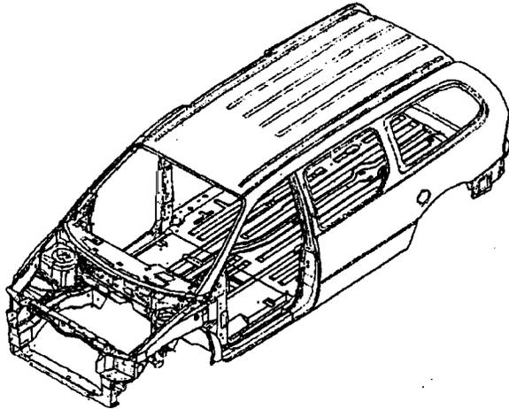
The main factors of the assembly process having impact on the BIW dimensional integrity are: (1) locating mechanisms in geometrical assembly stations, and (2) part-to-part interaction.
