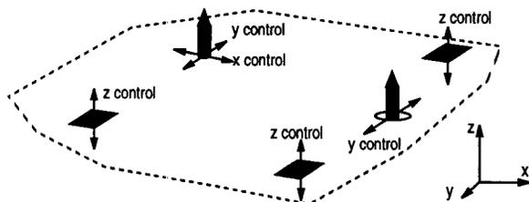
The 3-2-1 locating method utilizes fundamental geometry. Three points in space generate a plane, two points in addition to this first plane would generate a second plane perpendicular to it, while one final point generates a third plane perpendicular to the other two. Therefore, an xyz coordinate system would be generated
