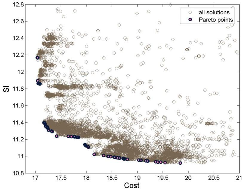
Fig. 7 Tradeoff between cost and sensitivity for  $\sigma_s=0.33$  mm
