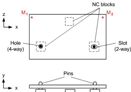
Fig. 2 Top and side views of the 3-2-1 fixture layout
