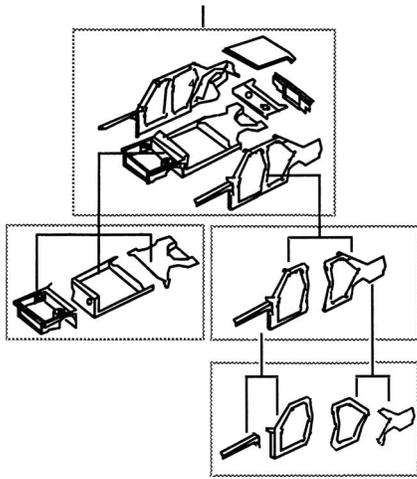
Fig. 1 Schematic of an automobile body structure assembly [1]
