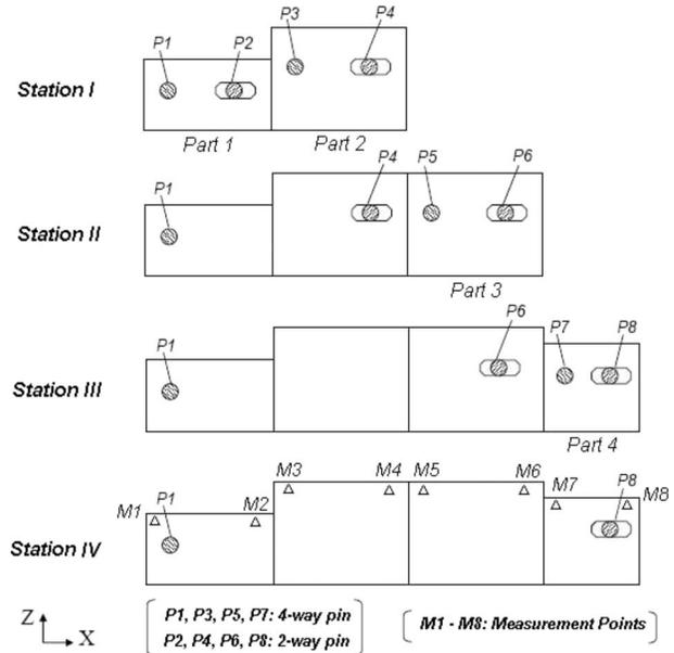
Fig. 6 Fixture layout in the rigid multistation assembly system
