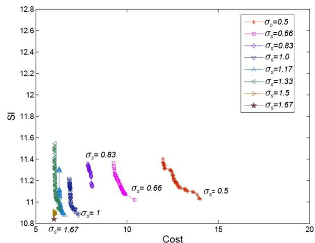
Fig. 9 Relation between cost and sensitivity for  $\sigma_s = 0.5-1.67$  mm
