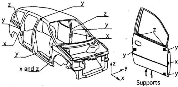
Figure 3. Layout of compensation points
