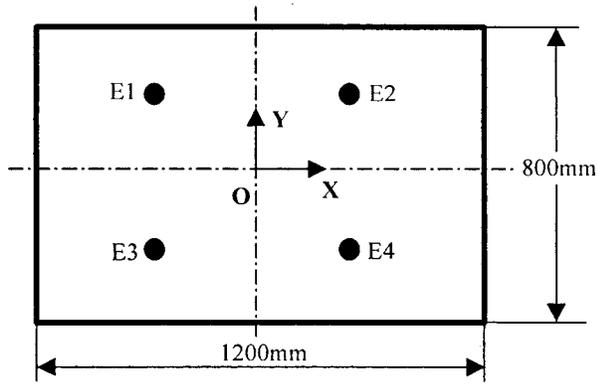
Fig. 2 An example of a sheet metal blank with end effector layout
