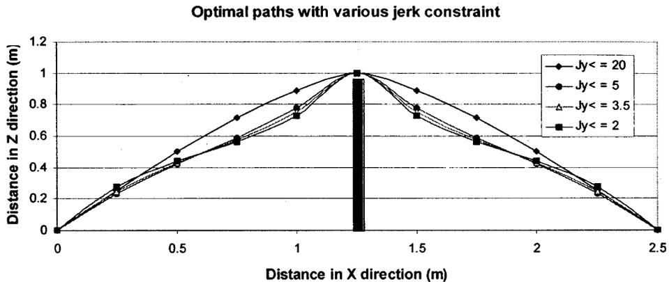
Fig. 15 Optimal trajectory with jerk constraint
