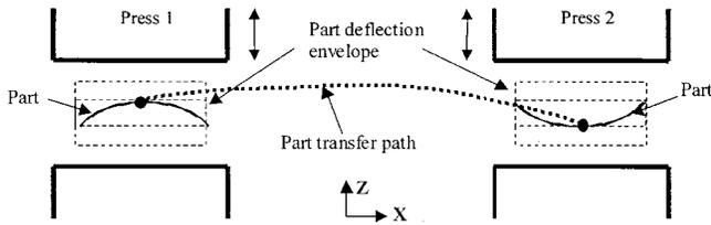
**Fig. 1 Schematic plot of compliant part transfer in a stamping line**
