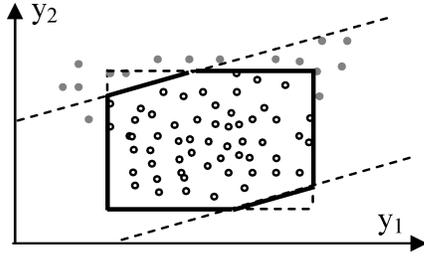
**Fig. 2.** An irregular tolerance region ( $|y_1 - y_2| \leq \Delta$  and  $L_i \leq y_i \leq U_i$ ) and a non-normal process.
