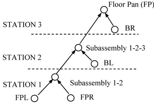
Fig. 6. Floor pan assembly tree.
