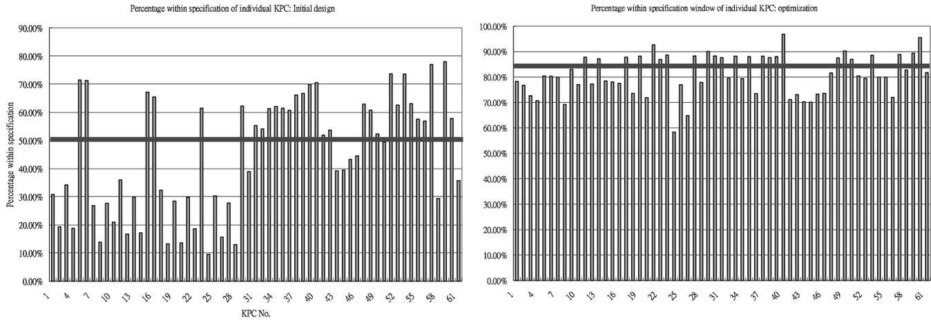
Fig. 8. Sixty one individual KPC’s yields: initial design (left) and optimal design (right).
