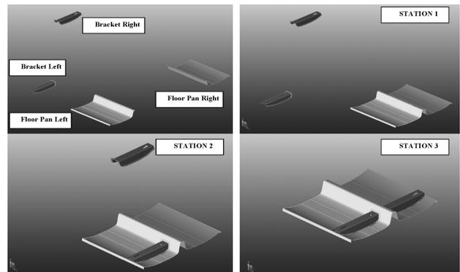
Fig. 5. A floor pan assembly.
