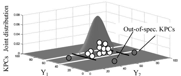
Fig. 1. In-spec. and out-of-spec. KPCs points.
