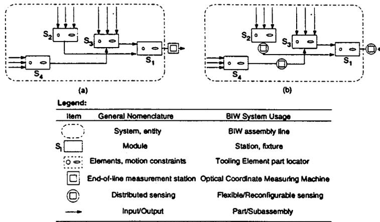
Fig. 1 Sensing approaches: (a) end-of-line sensing, (b) distributed sensing
