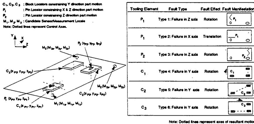
Fig. 2 Generic 3-2-1 fixture layout and corresponding failure mode fault manifestations
