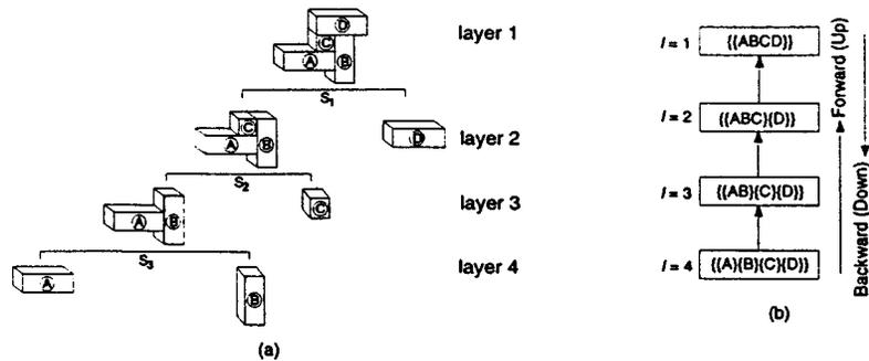
**Fig. 3 Assembly representation for optimization for (a) the example four-part widget assembly ( $S_1, S_2, S_3$  represent assembly stations), (b) state-transition representation (for each level  $l, \{\{\Theta\}\}$  is a partition representing assembly state, with element  $\{\theta_{ij}\}$  representing a subassembly or part)**
