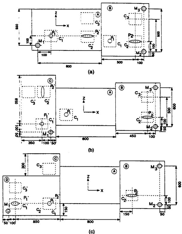
Fig. 5 Assembly part fixturing schematics for (a) station  $S_3$ , (b) station  $S_2$ , (c) station  $S_1$  ( $M_1$  are candidate sensor locations)
