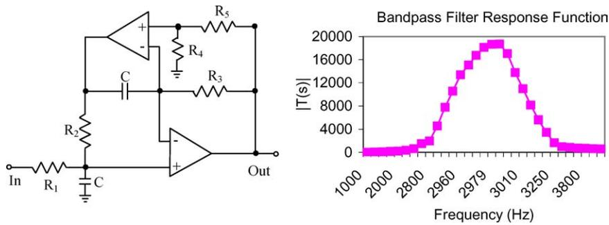
Figure 13. Dual-amplifier bandpass filter.
