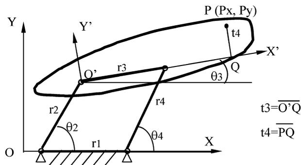
Figure 18. Four-bar mechanism.
