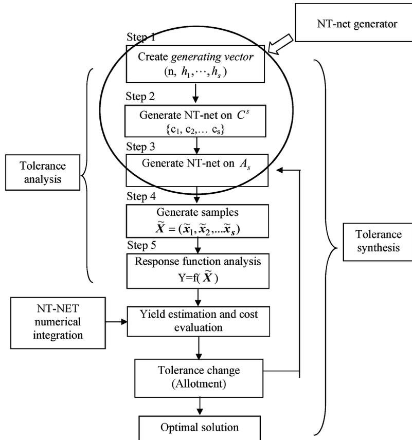
Figure 1. Flow chart of tolerance analyses/synthesis and simulation (the proposed NT-net replaces the Monte Carlo as the sample generator).
