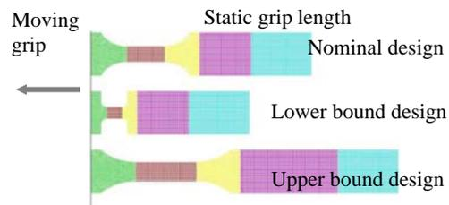
Figure 6. Models of specimen geometry variations. Moving grip length (to left of figure) and strain gauges omitted for brevity
