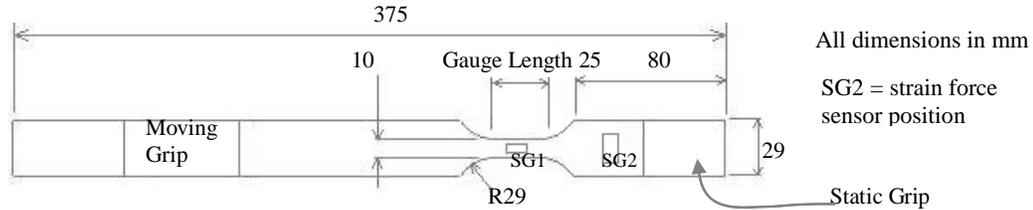
Figure 3. Specimen design for high velocity tensile test at 15 m/s
