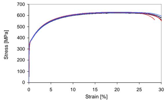
Figure 1. Engineering stress-strain test curves for steel tested in rolling direction (50mm gauge length[3]).
