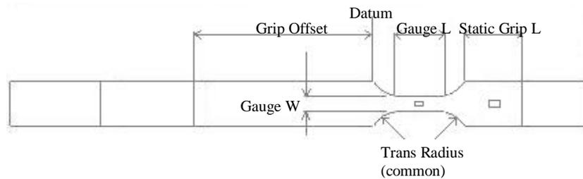
Figure 5: Definition of random geometry variables used in model
