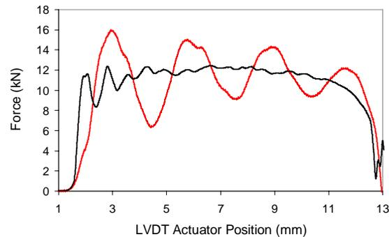
Figure 4. High speed test data generated at 15 m/s (strain rate  $\sim 600\text{ s}^{-1}$ , DAQ frequency set to 2.5 MHz)
